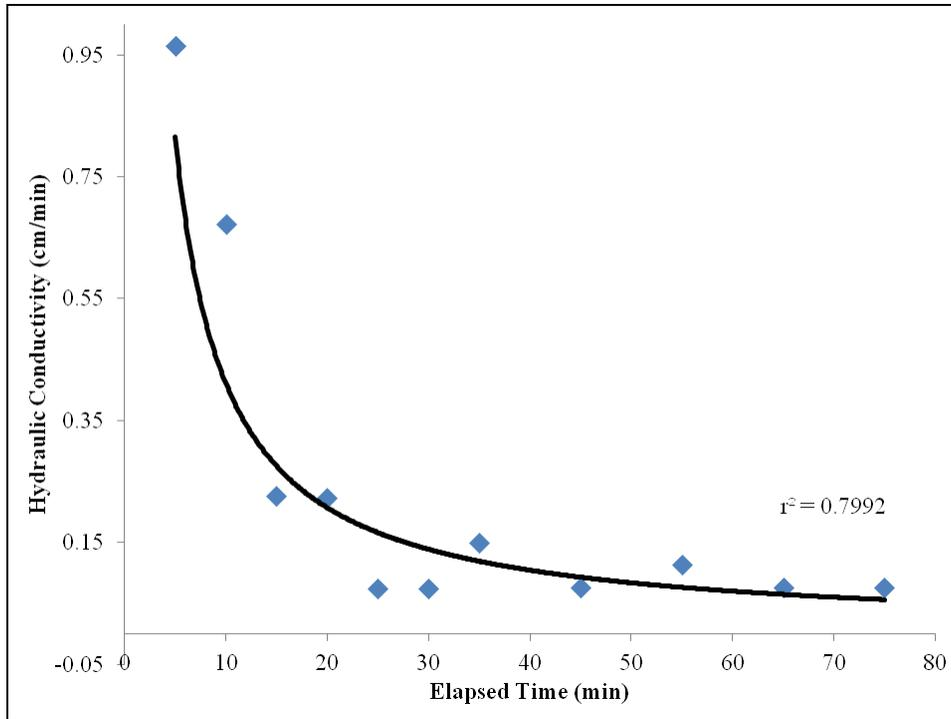
Figure B.13: Graph used to determine the hydraulic conductivity from the infiltrometer test performed in the area before windrow 1. The point at which the graph approaches a steady value is considered the hydraulic conductivity as demonstrated by the best fit line shown.
