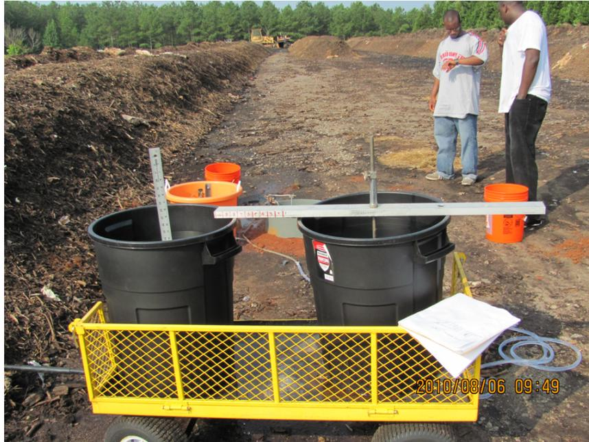
Figure B.11: Water was supplied to the rings by a set of water tanks and measured at a constant interval using rulers.
