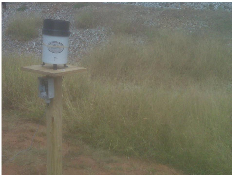
Figure B.6: Tipping bucket rain gauge used at the UGA Bioconversion Center to measure the amount of rainfall.
