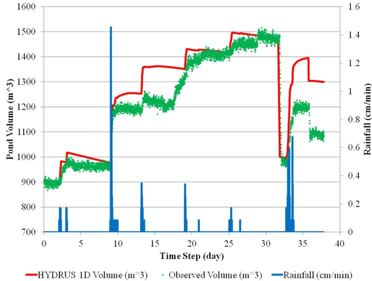
Figure B.1: Observed (green) and Predicted (red) values for pond volume based on rainfall (blue) during the calibration period using the HYDRUS 1D model.
