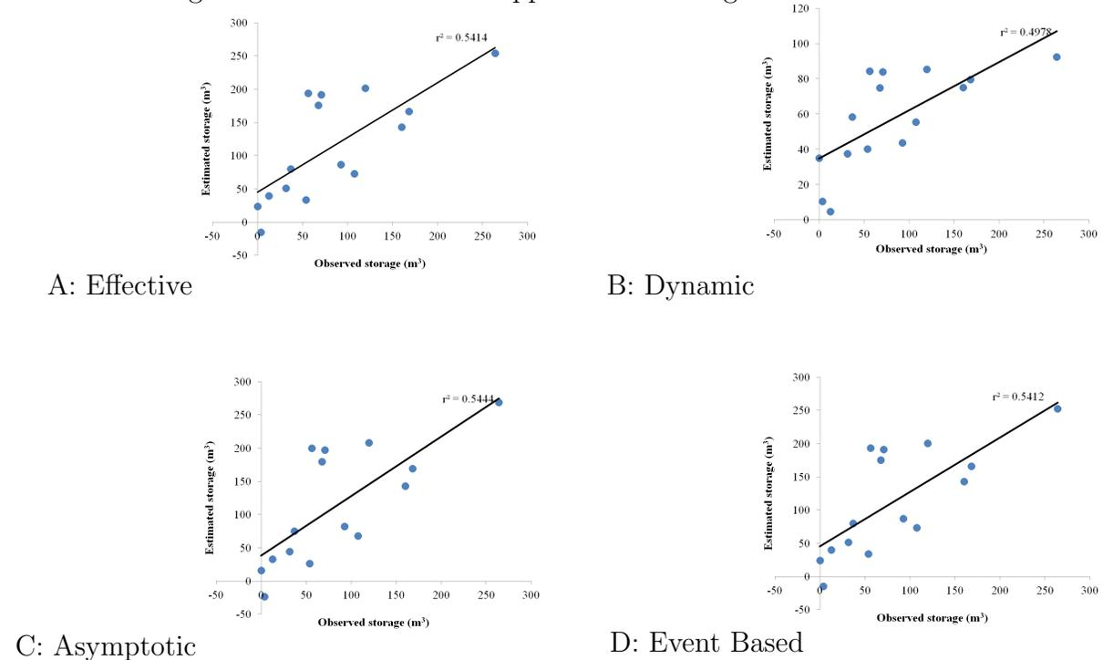
Figure 3.2: Graphs of the comparison of observed against the estimated volume of storage using the different curve number approaches.
