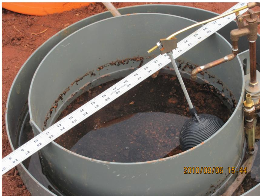
Figure B.12: As the water level in the ring increased, a float valve was used to keep the head of water constant.
