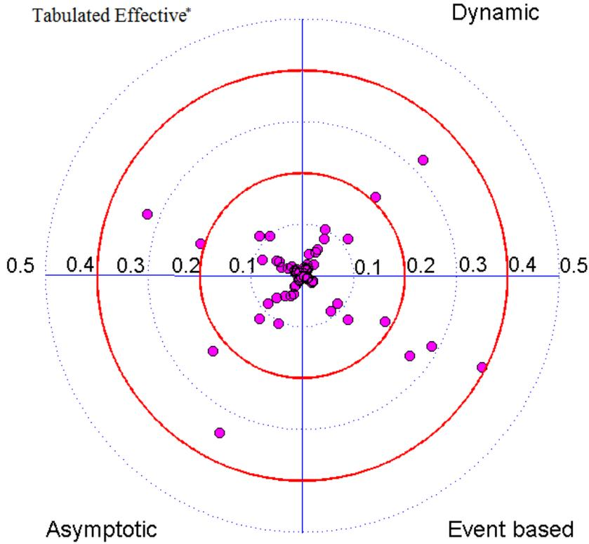
Figure 3.3: Fraction error from the calculation of runoff using the curve numbers based on NRCS tables, the dynamic approach, the asymptotic approach, and each individual event. \*As calculated by Kalaba et al. (2007)
