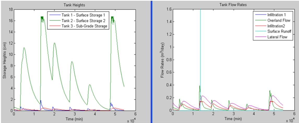
Figure 4.4: Matlab Simulink Graphs of flow rates and compartment heights. The above graphs show the expected relationship that as flow rates increase, the compartment heights properly respond with an increase as well. The parameters used were found using the Genetic Algorithm to search for the optimum parameters and discussed in Appendix B of Duncan (2012).
