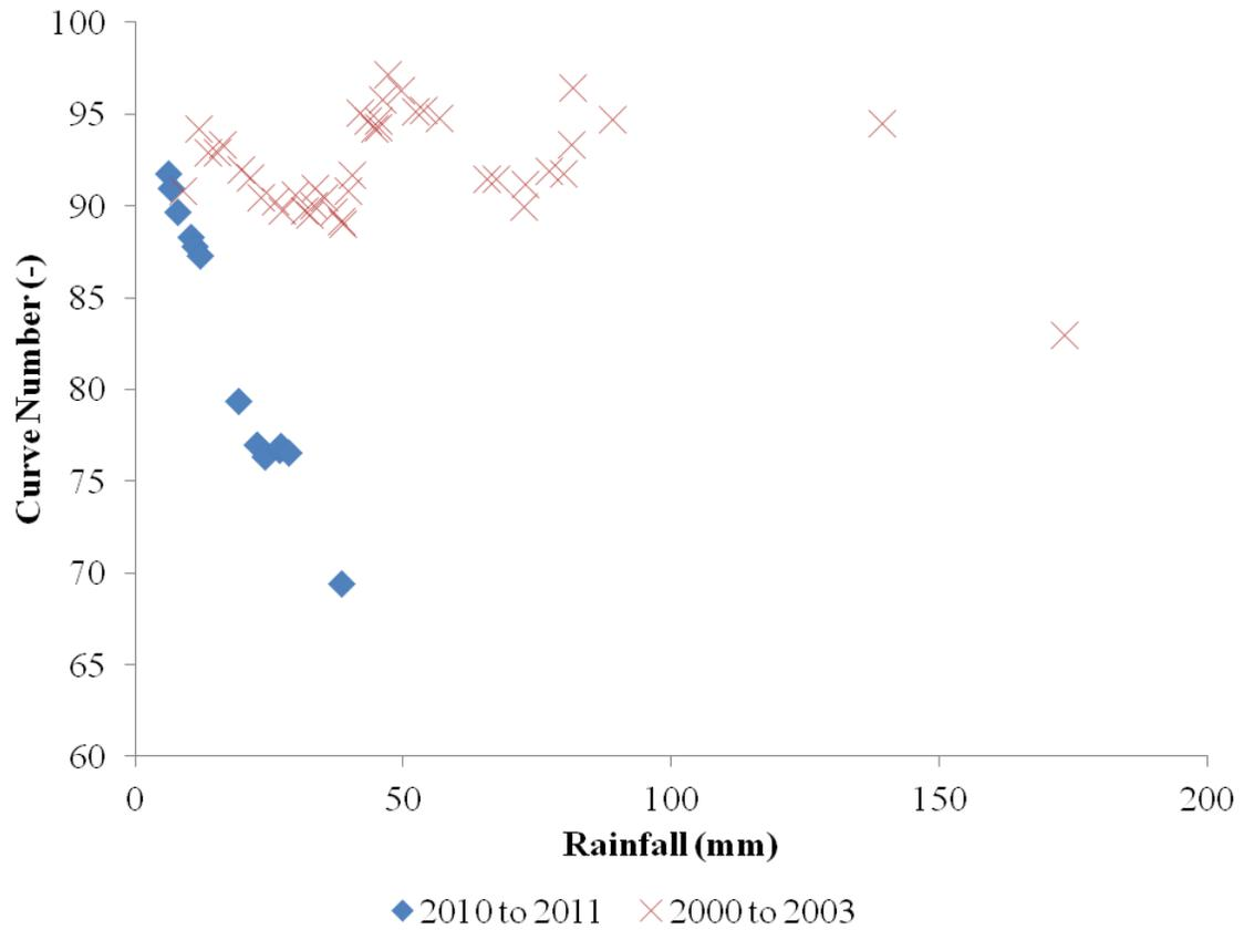
Figure 3.5: Calculated curve number versus rainfall for each event used to determine asymptotic curve numbers for the 2000 to 2003 storms (Tollner & Das, 2004) equal 96 and the 2010 to 2011 storms equal 70.5.
