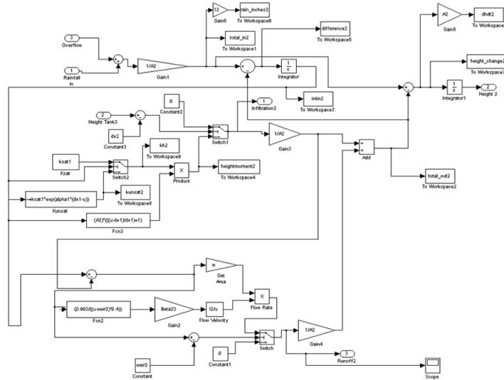
Figure B.18: Simulink Model of Compartment 2
