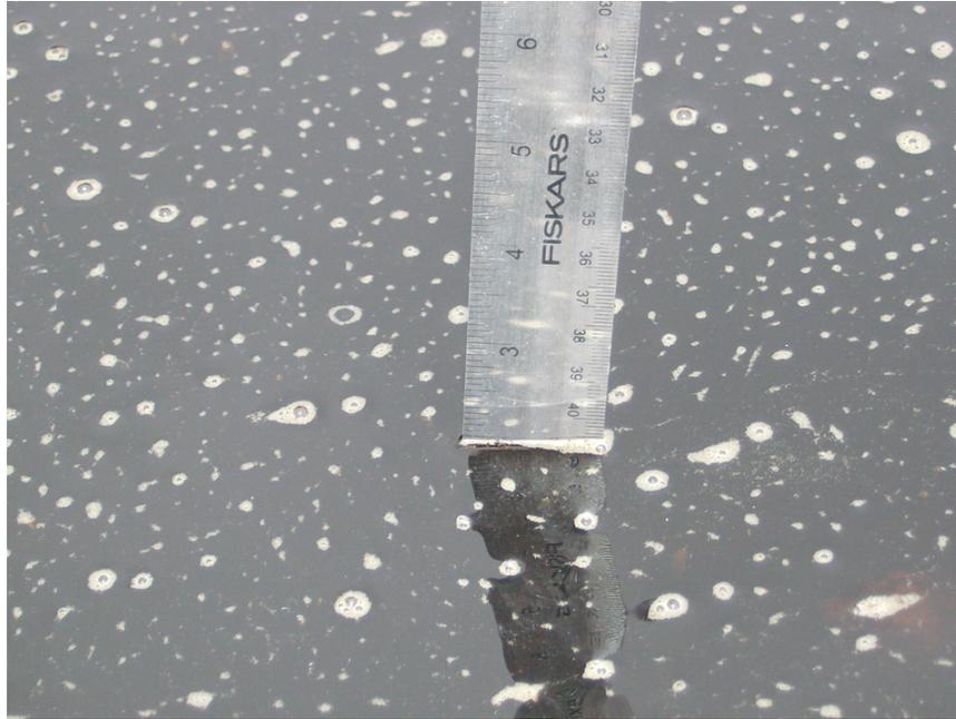
Figure A.5: A closer view of the height of storage that can occur due to machinery on the compost pad. Storage shown in the depression of the tracks was found 6 hours after the previous storm.
