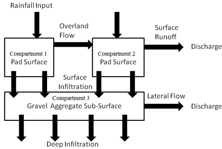
Figure B.5: Storm water dynamics of porous pavements using the three compartment system used to analyze rates of surface runoff, infiltration, and lateral flow.
