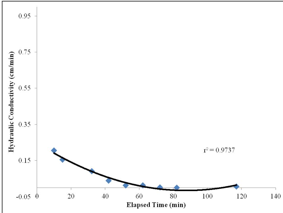
Figure B.15: Graph used to determine the hydraulic conductivity from the infiltrometer test performed in the area between windrows 4 and 5. The point at which the graph approaches a steady value is considered the hydraulic conductivity as demonstrated by the best fit line shown.
