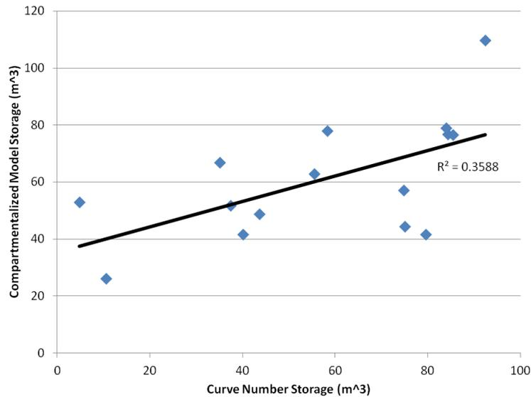
Figure 4.5: Comparison of the calculated volume of storage using the compartmentalized dynamic model and the curve number method.
