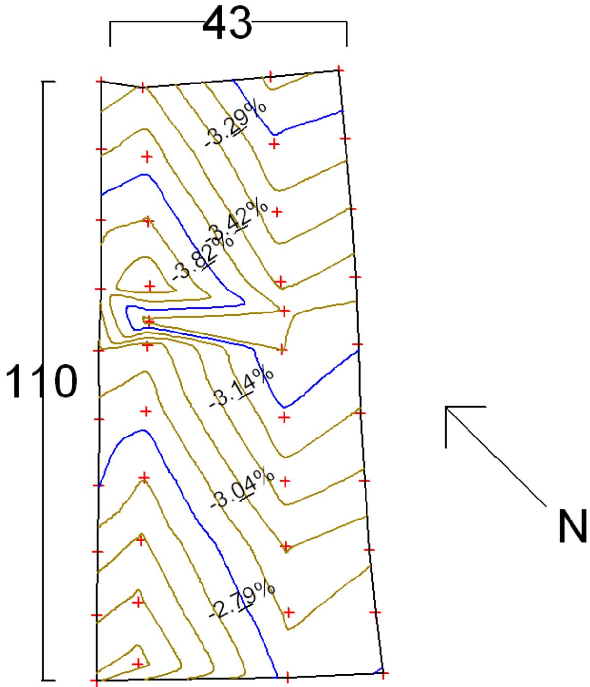
Figure A.1: Topography of the UGA Bioconversion Center Composting Pad. The direction of slope shown is the percent slope. The units for the length and Width of the Pad are in meters.
