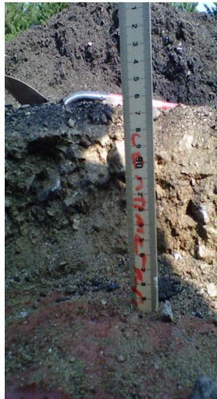
Figure B.4: Profile view of the sub-surface gravel/sand aggregate layer of the compost pad. This layer extends from the surface of the compost pad down to the compacted clay layer.
