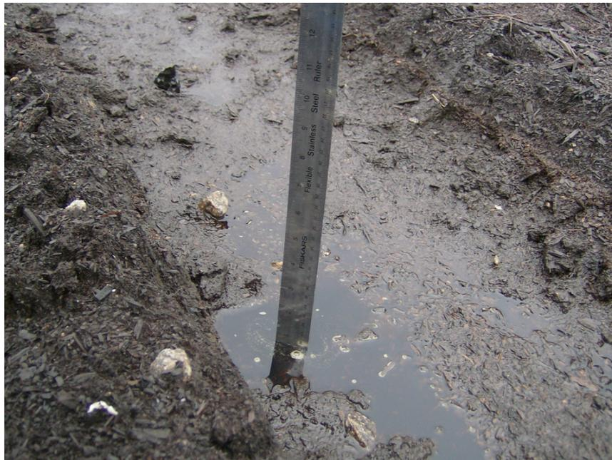
Figure A.4: Image of the height of storage that can occur due to machinery on the compost pad. Storage shown in the depression of the tracks was found 6 hours after the previous storm.
