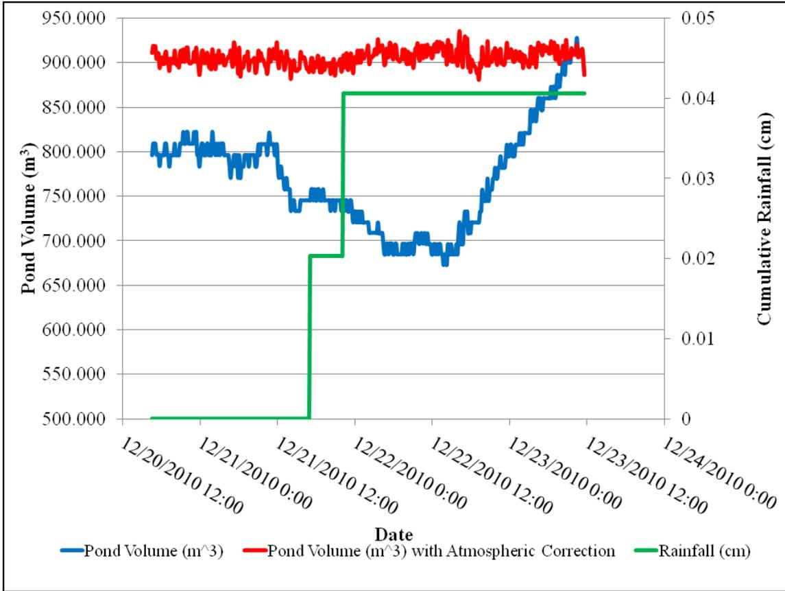
Figure B.8: A comparison of the error that can occur from the pond level logger when the impact of barometric pressure is not accounted for. During the rainfall event, changes in atmospheric pressure caused the logger to underestimate the level in the pond.
