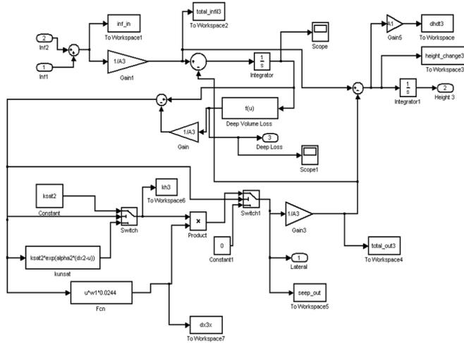
Figure B.19: Simulink Model of Compartment 3
