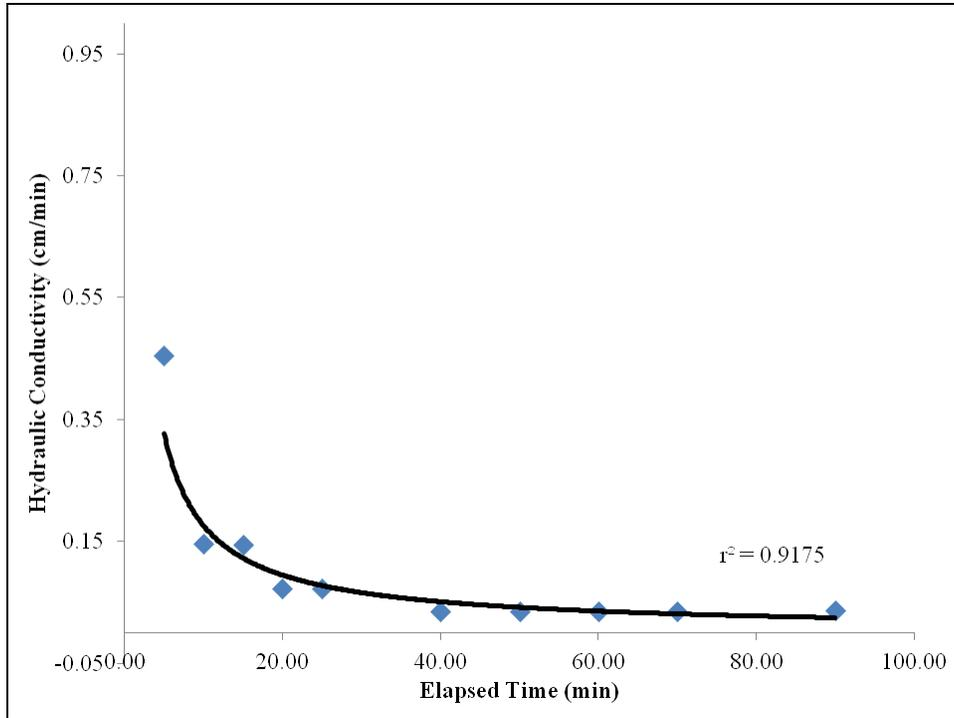
Figure B.14: Graph used to determine the hydraulic conductivity from the infiltrometer test performed in the area between windrows 2 and 3. The point at which the graph approaches a steady value is considered the hydraulic conductivity as demonstrated by the best fit line shown.
