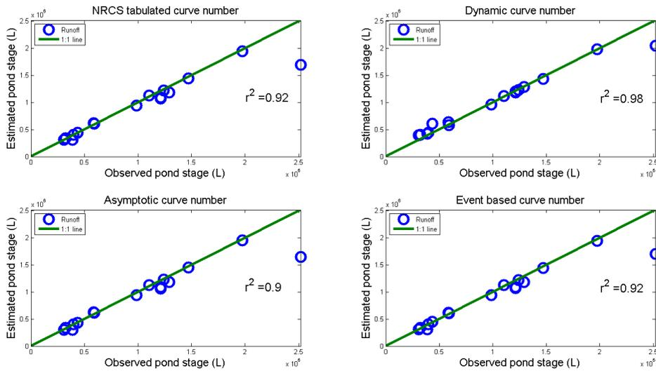
Figure 3.4: Estimated pond stage from the four different curve number methods compared to runoff observed in 2010 to 2011.
