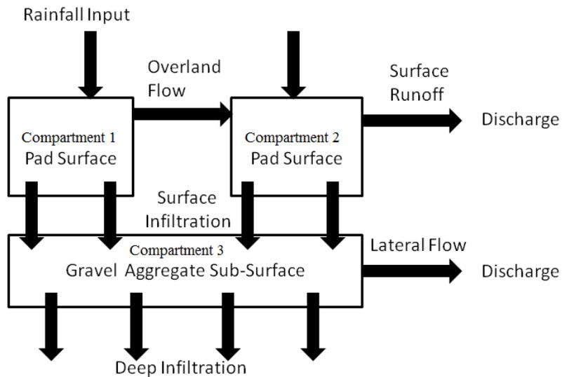
Figure 4.2: Storm water dynamics of porous pavements using the three compartment system used to analyze rates of surface runoff, infiltration, and lateral flow.
