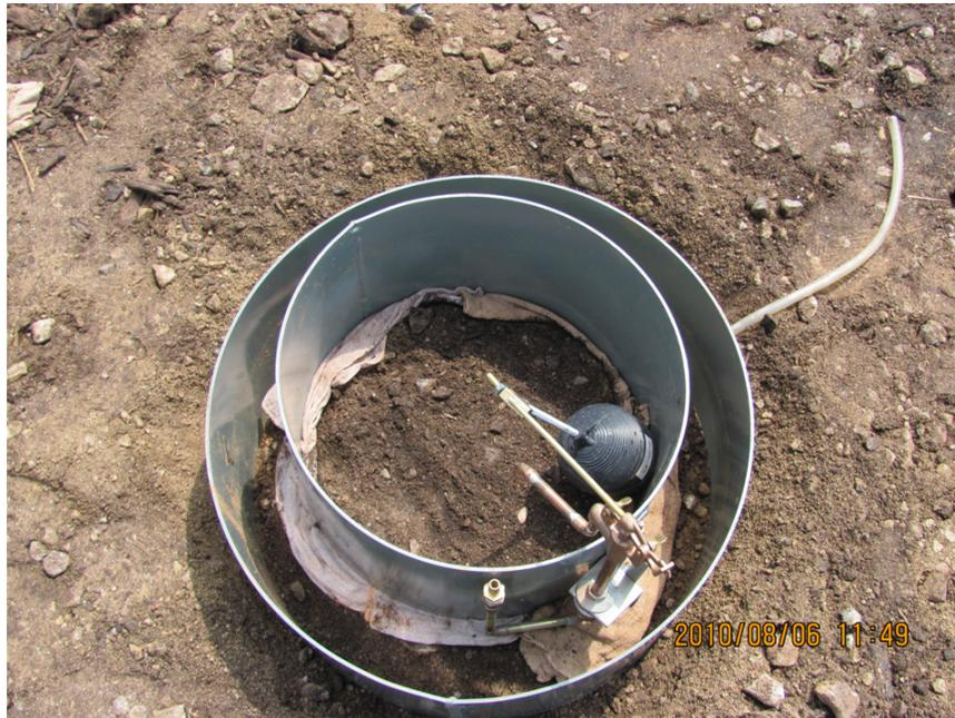
Figure B.9: After a proper location was found and extra debris was cleared away, the rings were placed in the ground at a depth that would prevent lateral loss.
