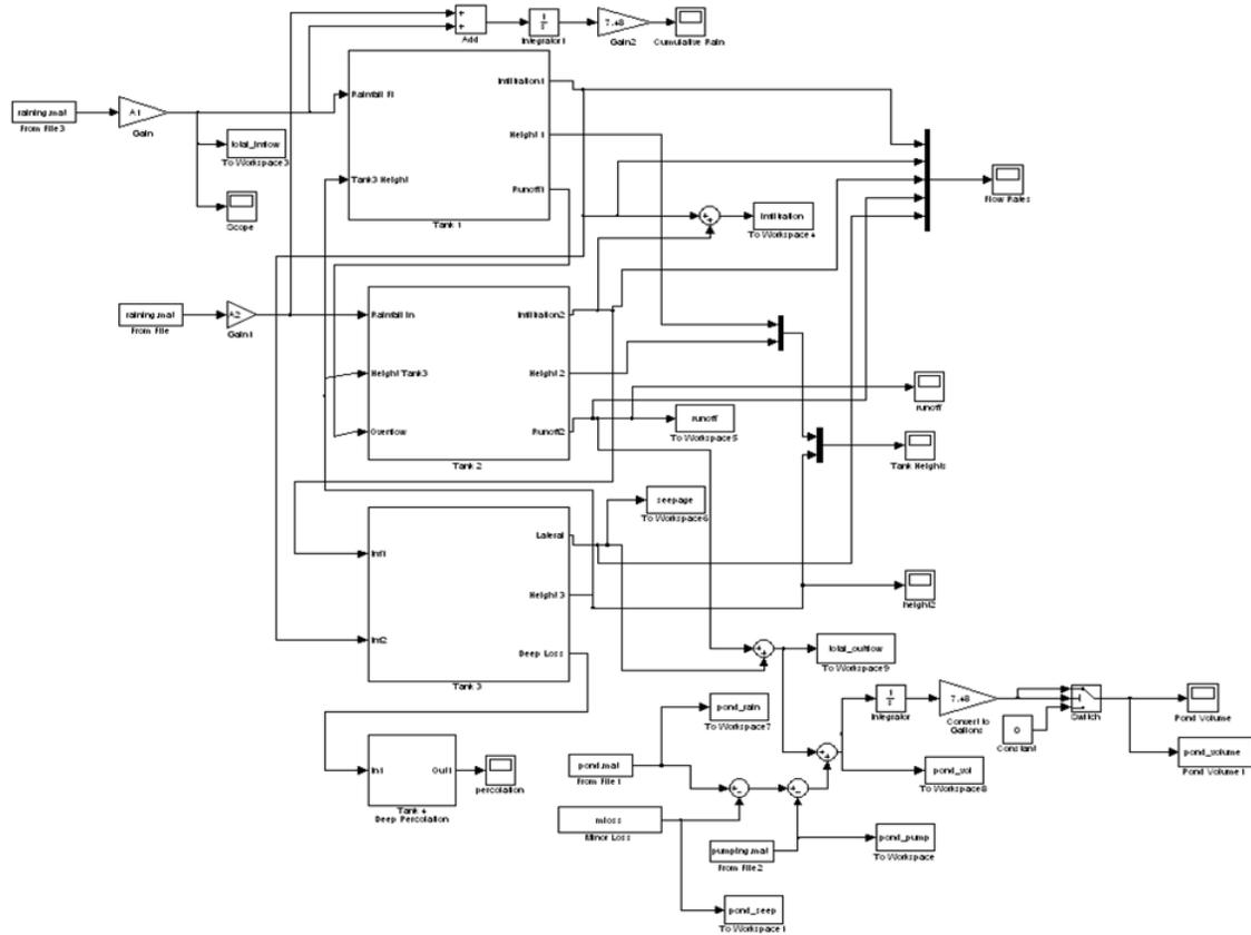
Figure B.16: Full compartmental model built in Simulink. The rainfall input as well as all variables are read from the Matlab workspace. At the end of the model, the rates of infiltration, runoff, storage for each tank and the resulting pond volume are exported to the Matlab workspace.
