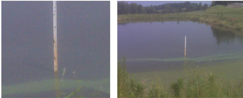
Figure B.7: (Left) Staff gauge used to determine the reference height in the collection pond. B. (right) Full view of the collection pond used to collect runoff from the compost pad.
