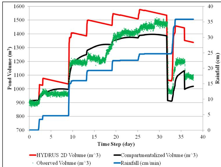
Figure 4.3: Observed (green) pond stage compared to the trend of estimated pond stage by the Compartmentalized Dynamic Model (black) and HYDRUS 2D Model (red) values for pond volume based on the cumulative rainfall (blue) using from December 23, 2010 to January 30, 2011.
