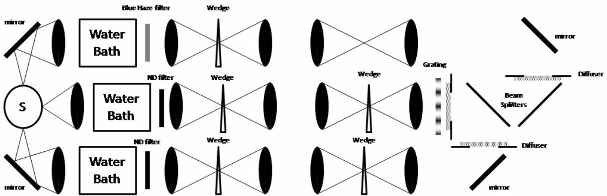
Figure 1. A diagram of the optical system used in this experiment. Channels 1 and 2 (lower and middle respectively) were used in all three conditions, however, Channel 3 (upper) was only active during the visibility experiment.
