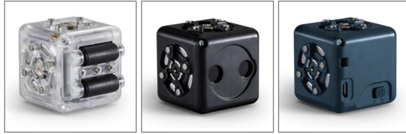
Figure 2. Drive Actor (left), Distance Sensor (middle), and battery (right).
