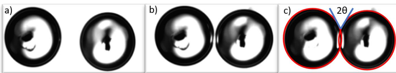
Figure 10: Membrane formation using the droplet interface bilayer technique. a) Initially, the droplets are apart forming only the monolayers. b) Approaching the droplets leads to the spontaneous membrane formation. c) The membrane is formed, and the two droplets are separated by a contact angle 2\theta .
