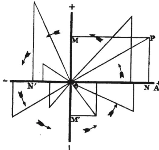
Figure 9. De Morgan's rotated angles and sine and cosine as projections.
