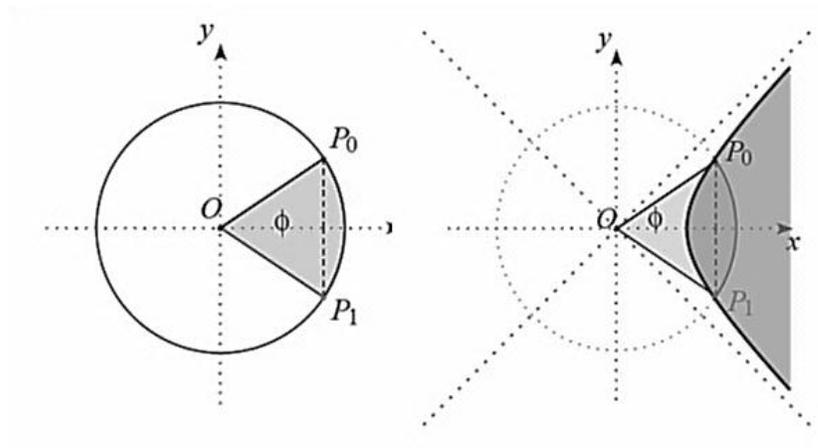
Figure 5. Sector area as the argument for circular and hyperbolic trigonometric functions.
