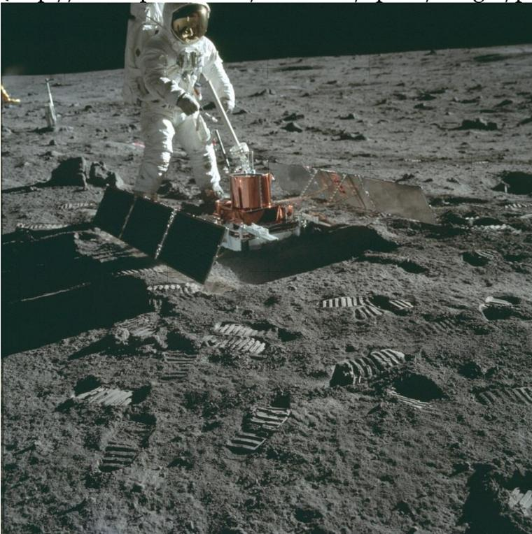
Figure 1.3. Astronaut deploying seismic experiment equipment
