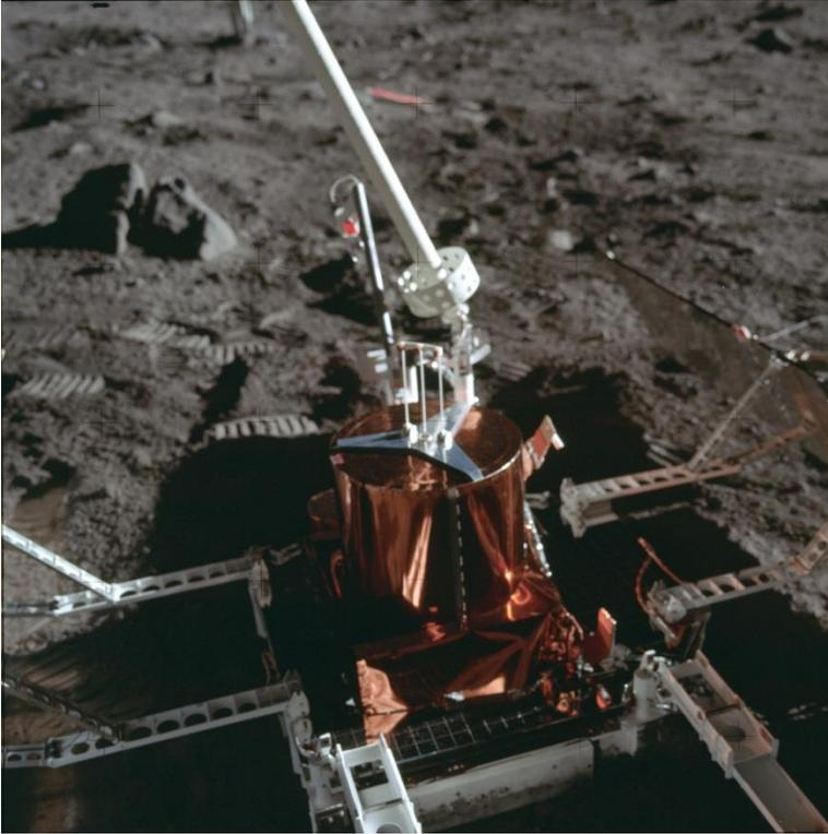
Figure 7.16. Seismic experiment equipment remaining at Tranquility Base
