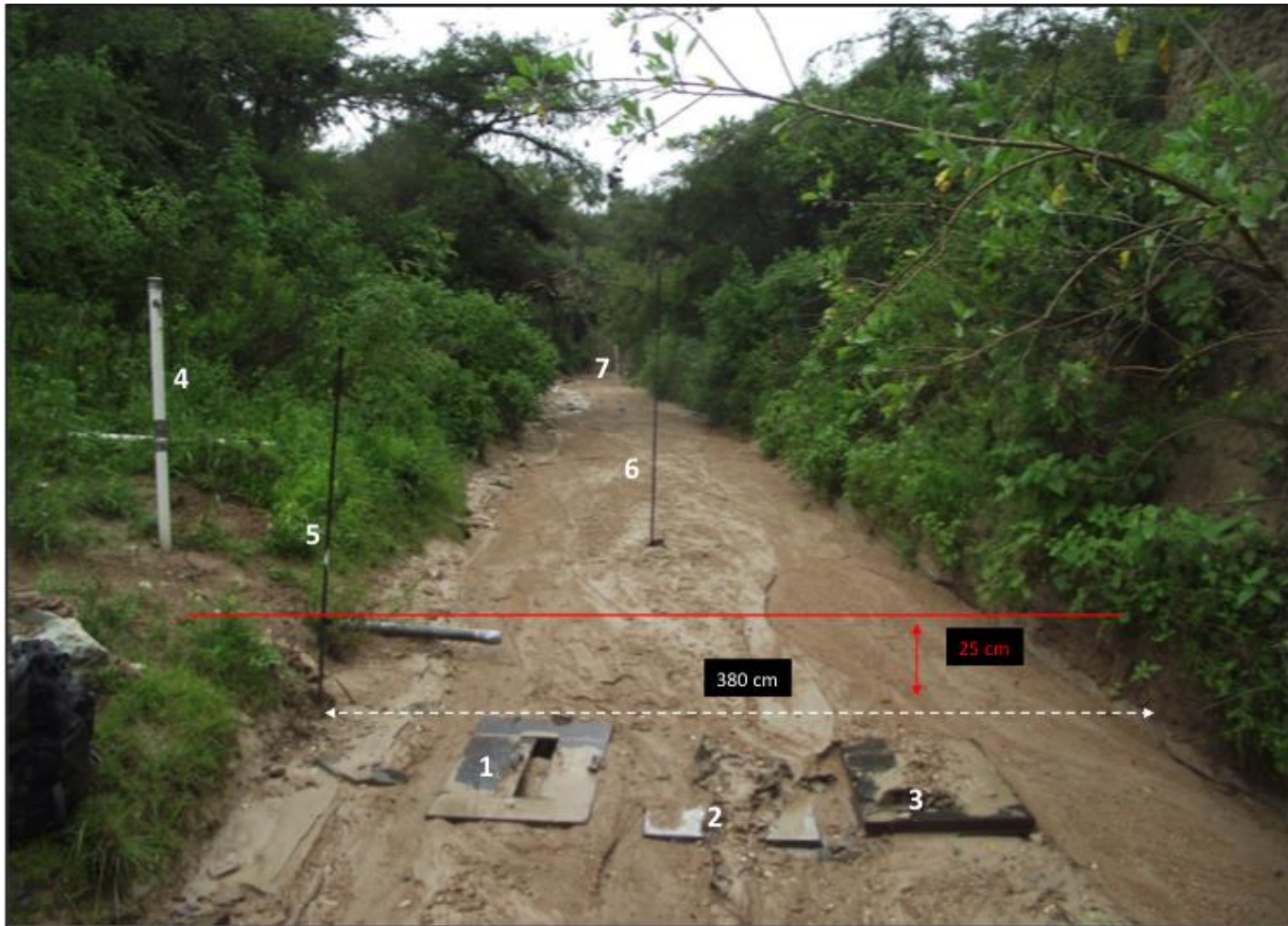
Figure 2.5. Monitoring station of Barranca Sandage. The monitoring station includes: three bedload traps (denoted by numbers 1-3), Odyssey stage recorder (4), staff gauge (5) and peak stage recorders in distance (6-7) (one of them has been removed already). The red line indicates the location of bankfull flow.
