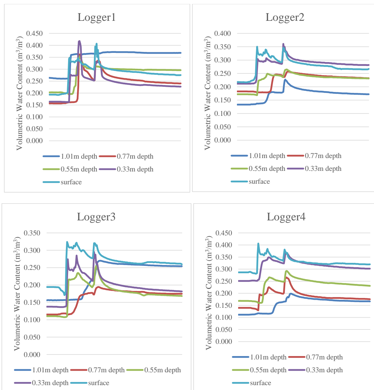
Figure 2.27. Soil moisture sensor data (volumetric water content) from Storm 5, over a 50-hour period starting October 14, 2014, at midnight
