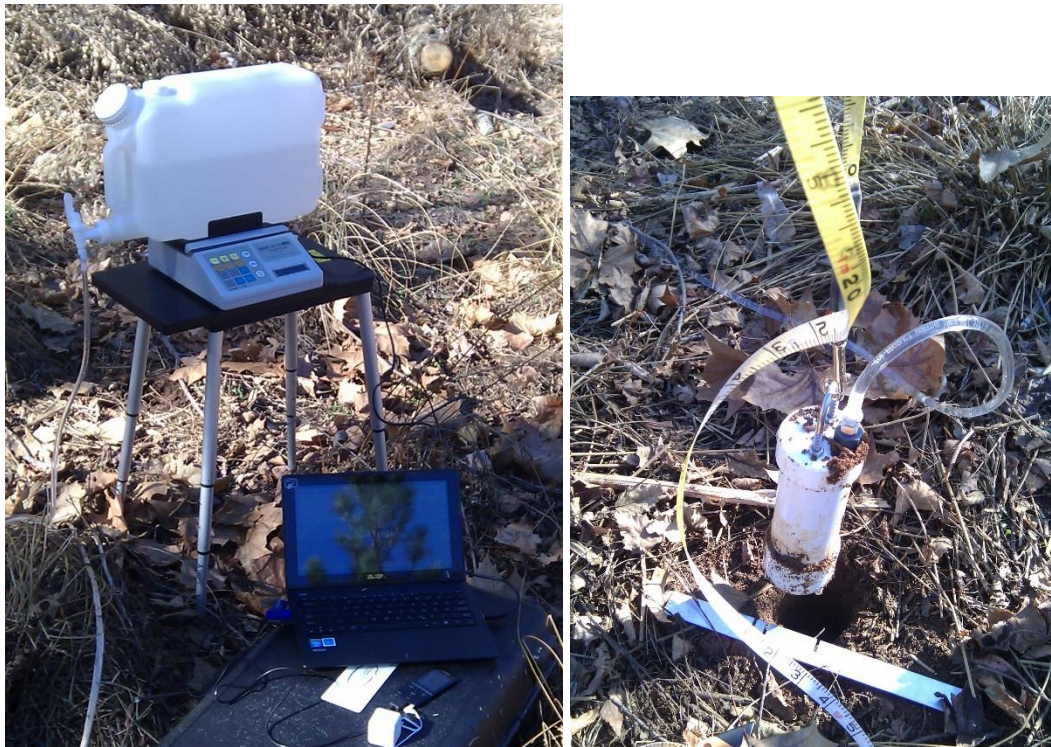
Figure 2.6. Permeameter setup in garden, with close-up of capsule module. The capsule is lowered into an auger hole, and water flows out of it at a rate determined by the infiltration ability of the underlying soil.
