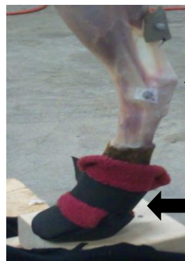
Figure 2.1: Pictures of the modified Oxford Knee Rig that characterize its motion, how the vertical bolt running through the ischial tuberosity and a horizontal bolt through the sacroiliac joint of the ilium were used to attach the hemi-pelvis to the OKR while preserving the coxofemoral joint, and the dog boot that preserved the hock.
