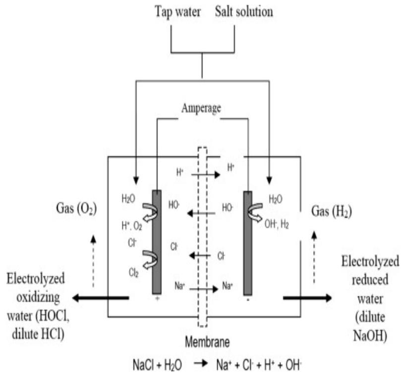
Fig. 2.1: Schematic of electrolyzed water generator and produced compounds
