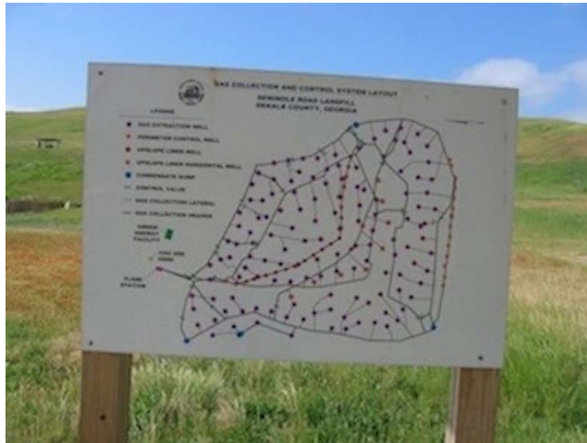
Figure 6-Map detailing LFG wells and pipelines
