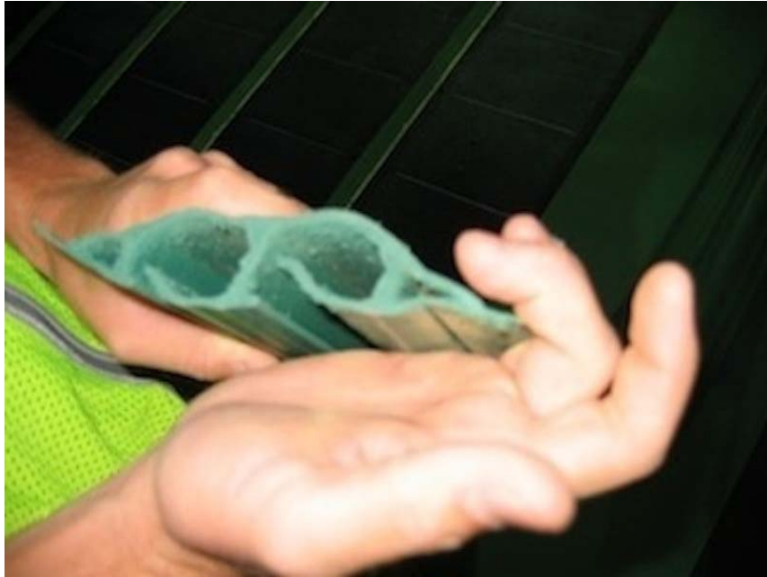
Figure 22-A close-up of the wire races that run the length of the panels to protect the wires.
