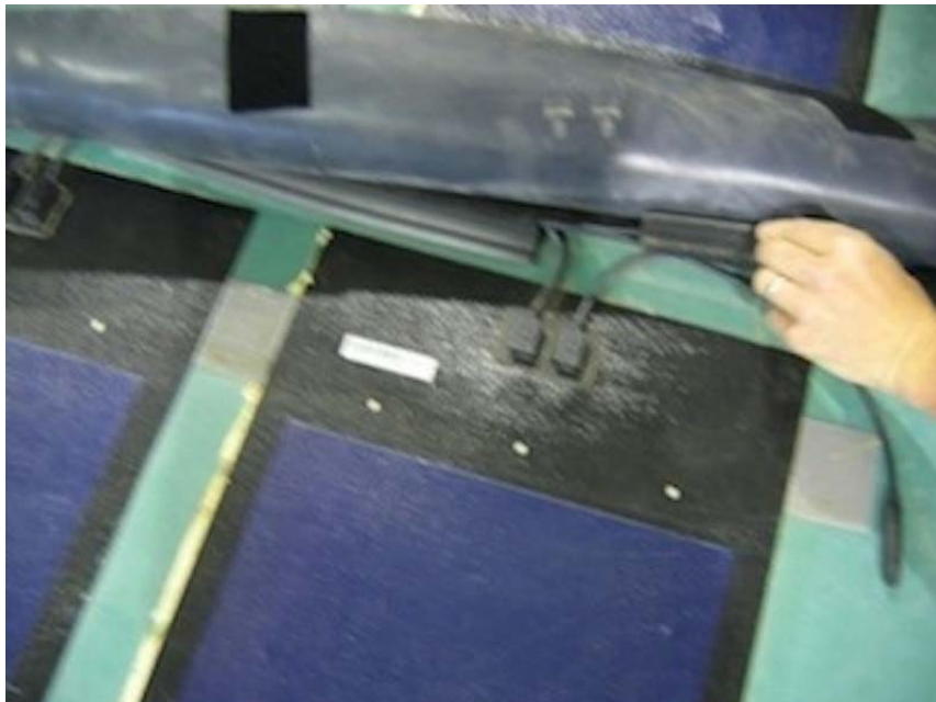
Figure 21-A close-up of the panel wiring. The wiring is protected by wire races.
