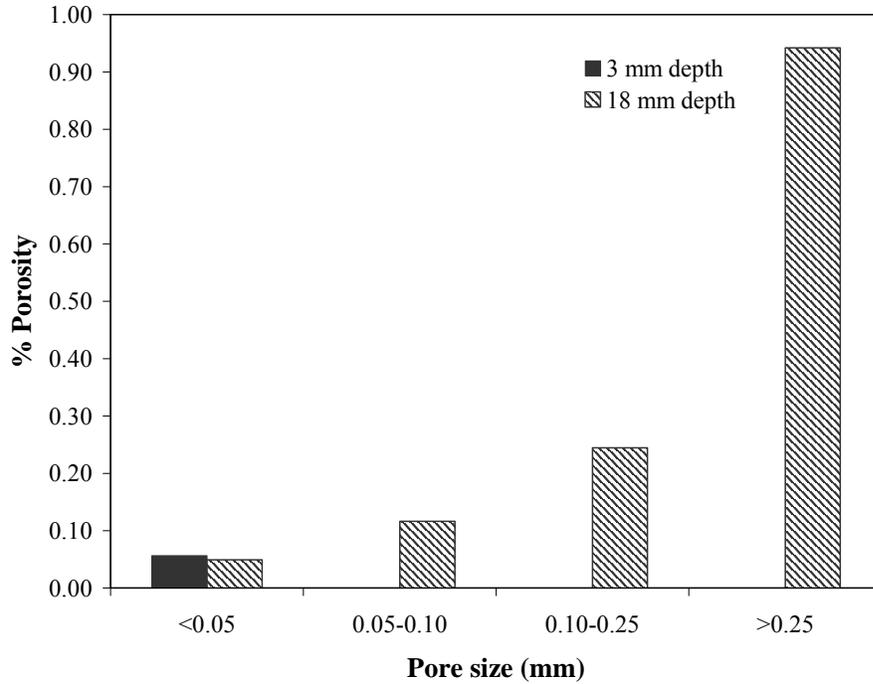
Figure 3-9. Pore size distribution at two depths in the biomat-affected soil at Site E. The biomat at this site is 3 mm thick. No pores >0.05 equivalent diameter were present in the biomat.
