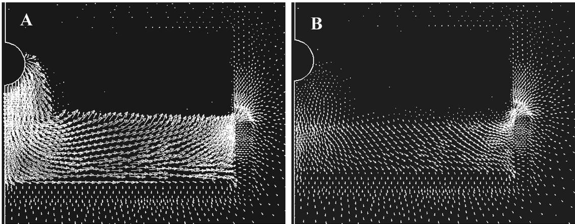
Figure 4-5. Velocity vectors for dispersal field in clay loam soil with equal  $K_s$  values for trench bottom and sidewall biomat. A-Dosing time is 2000 h with the highest ponding depth (11.2 cm). B-Resting period between doses with low flow.
