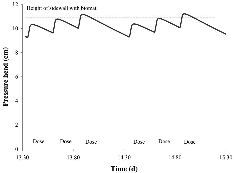
Figure 4-2. Pressure head (cm) of dispersal field in clay loam soil with equal trench bottom and sidewall  $K_s$ .
