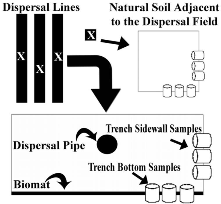
Figure 3-1. Method of sampling for biomat-affected soil and unaffected soil.
