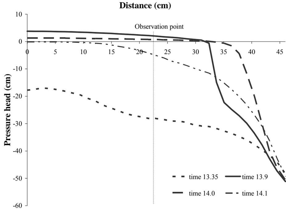
Figure 4-9. Pressure heads (cm) for different times (d) at the trench bottom of the dispersal field in sand soil.
