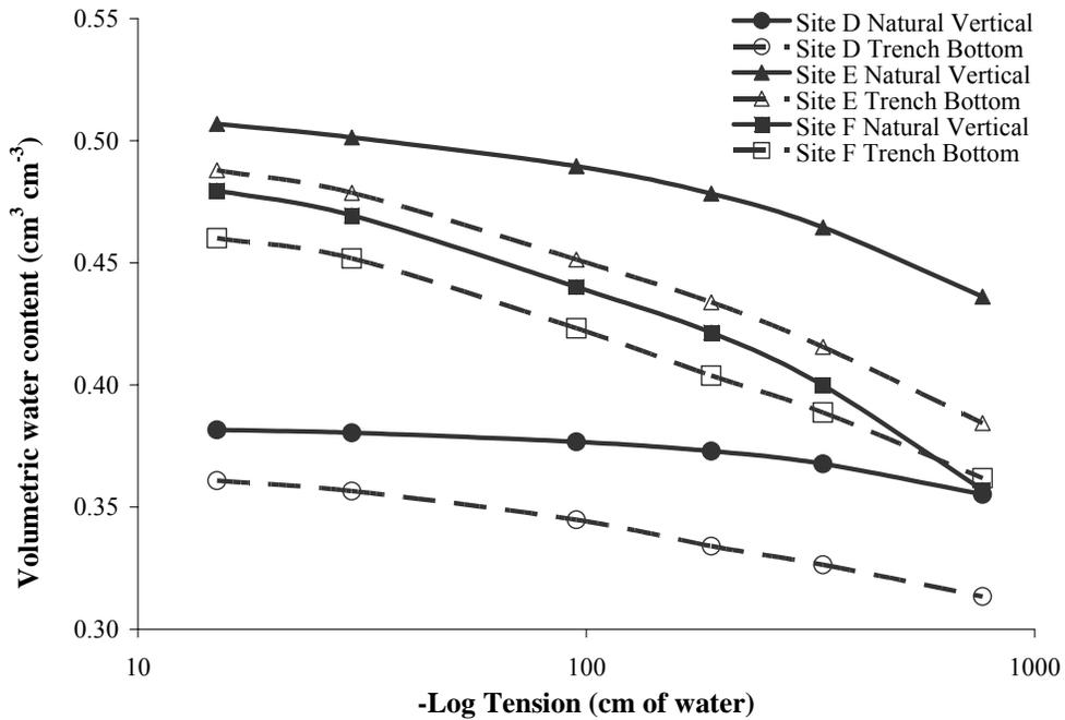
Figure 3-10. Soil-moisture release curve of natural vertical soil and trench bottom soil of Site D, E, and F. The volumetric water content of each site compared to the tension (log).
