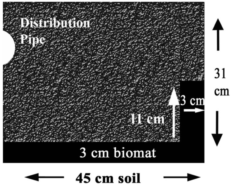
Figure 4-1. Half the dispersal trench used for model simulations.
