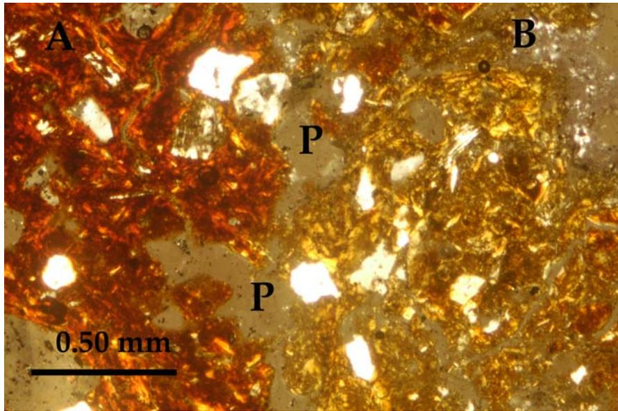
Figure 3-7. Thin-section of trench bottom samples from Site E. A-Red soil unaffected by wastewater application. B-Red Fe oxide coatings removed due to Fe reduction in the soil with presence of wastewater. P=pore, partially crossed polars.
