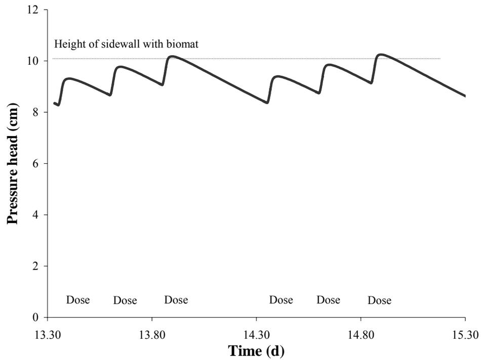
Figure 4-7. Pressure head (cm) of dispersal field in clay loam soil with 2 times the trench sidewall biomat  $K_s$  than the trench bottom biomat  $K_s$ .
