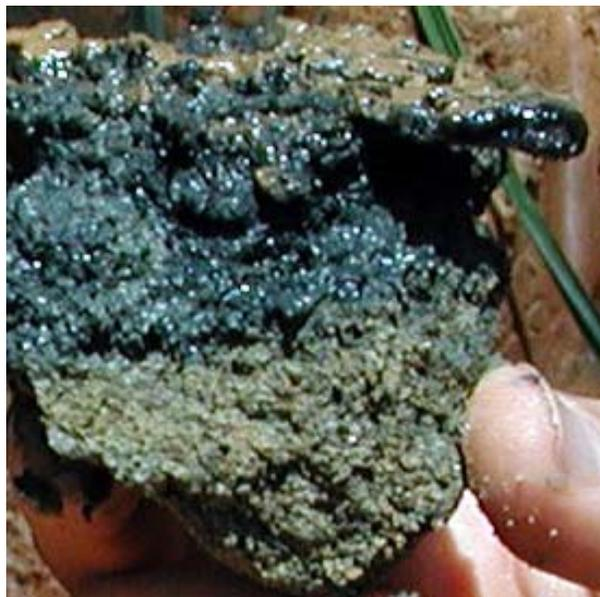
Figure 3-4. Biomat from the trench bottom of Site A. Thickness of dark material is about 3 cm.
