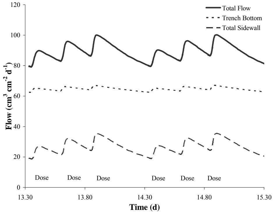
Figure 4-3. Total system, trench bottom, and sidewall flow of dispersal field in clay loam soil with equal trench bottom and sidewall  $K_s$ .
