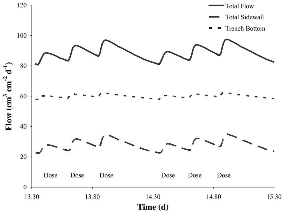
Figure 4-6. Total system flow, sidewall flow, and trench bottom flow of dispersal field in clay loam soil with 2 times the trench sidewall biomat  $K_s$  than the trench bottom biomat  $K_s$ .
