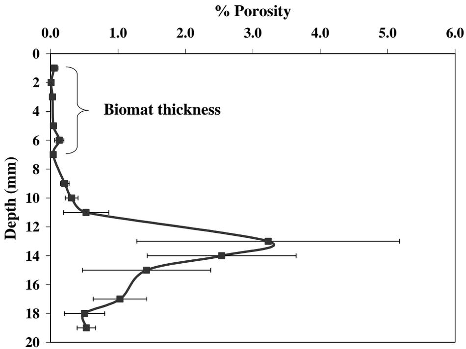
Figure 3-2. Percentage porosity with depth of polished block sample from Site C. The biomat was estimated to be 7 mm thick at this site.
