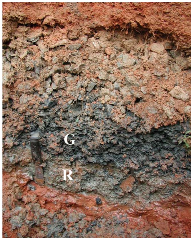
Figure 3-6. The trench bottom of Site E with biomat-coated gravel (G) and reduced soil below the biomat-affected soil (R).
