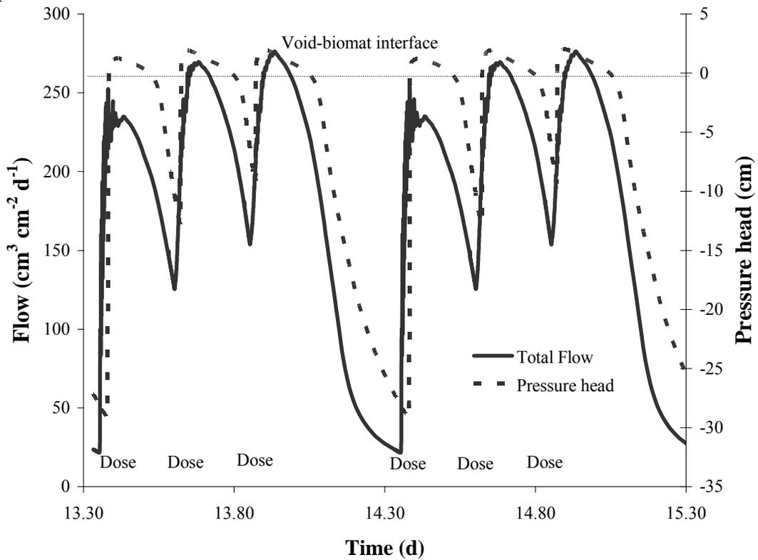
Figure 4-10. Total flow (cm/day) and pressure head (cm) of the dispersal field in sand-textured soil.
