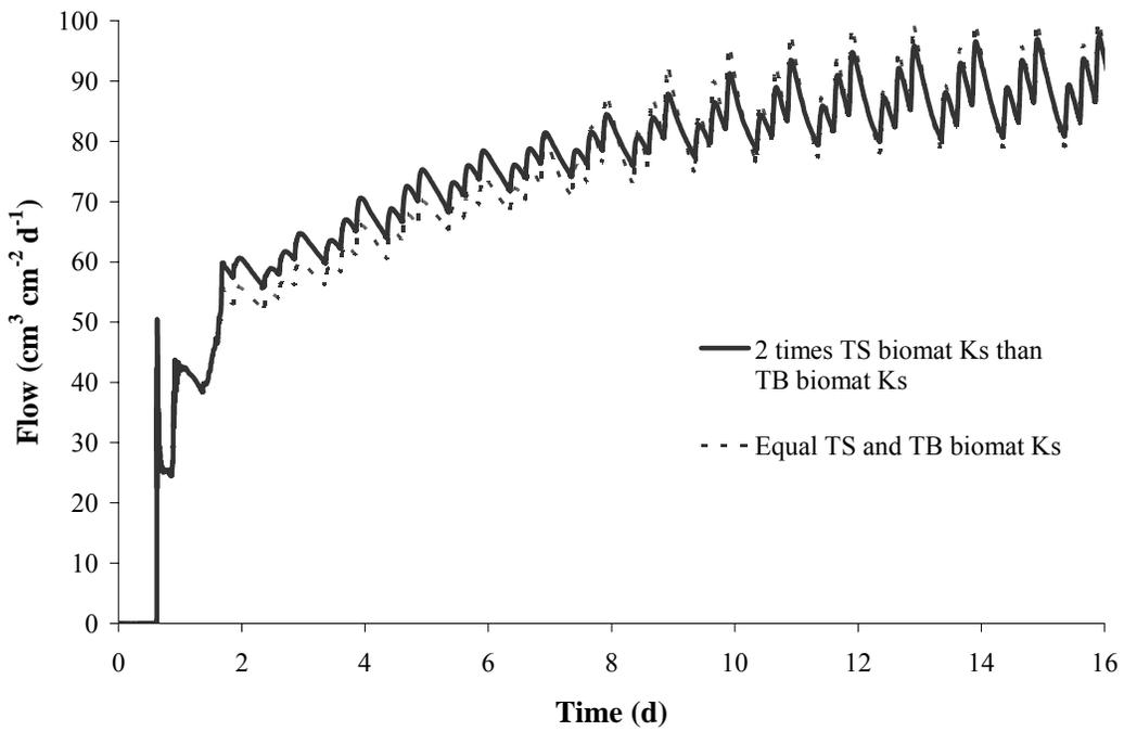
Figure 4-8. Total flow from time zero to steady state (13 d) for the clay loam flow simulations.
