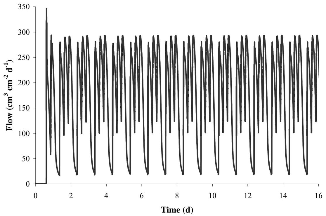
Figure 4-11. Total flow for time zero to steady state (2 d) representative of both sand models.
