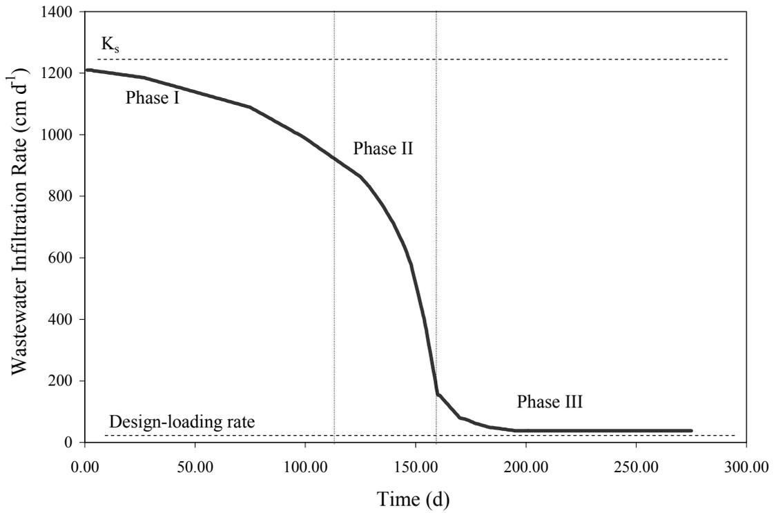
Figure 2-1. Infiltration rate reduction with time under wastewater application: Adapted from Thomas et al., 1966.
