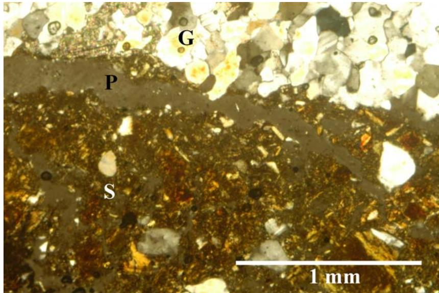
Figure 3-3. Thin-section of gravel piece above soil. Note crack between soil and overlying gravel that may indicate slight disturbances during sampling. G=gravel; S=soil; P=pore. Partially crossed polars.
