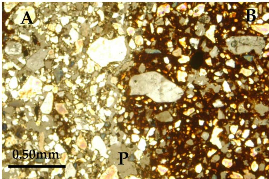
Figure 3-8. Reduction of Fe and Mn in trench bottom thin-section from Site D. A-gray soil reduced from Fe reduction and loss under the influence of wastewater. B-soil unaffected by wastewater. Note the closer placing of grains and less fine material in the gray zone. P=pores, partially crossed polars.
