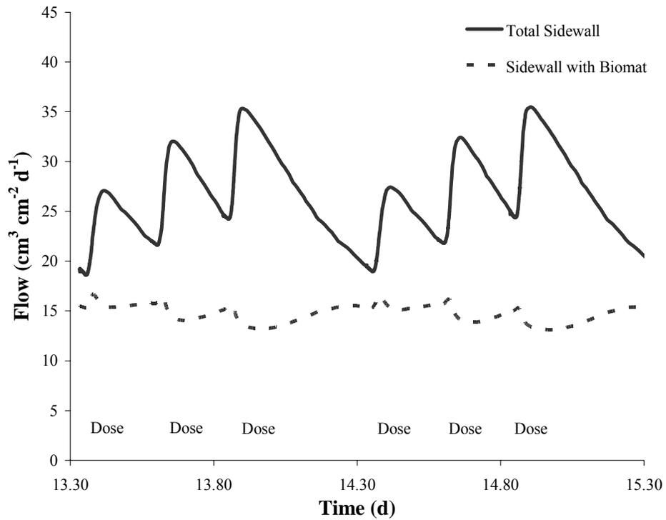
Figure 4-4. Total sidewall and sidewall with biomat flow of dispersal field in clay loam soil with equal trench bottom and sidewall  $K_s$ .
