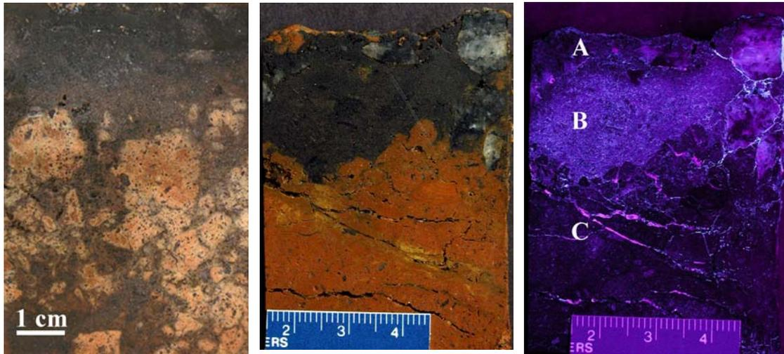
Figure 3-5. Polished blocks of trench bottom samples; Left-plane light image from Site E Middle-plane light image from Site C, Right-same view as left except photographed under UV light. A-biomat B-organic material coated grains C-subsoil. Scale in cm.
