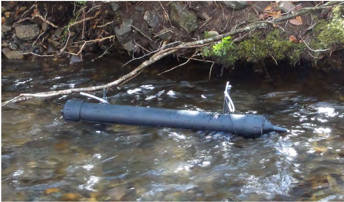
Figure 2.5. Suspended Sediment Sampler installed in Ball Creek above baseflow.
