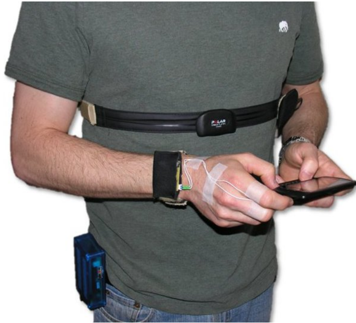
Figure 5.3: Stress monitoring using intrusive sensors. Courtesy of J. Choi [2010].
