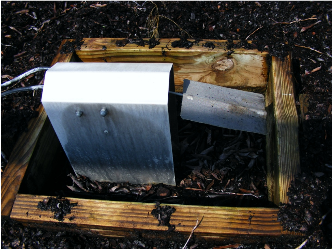
Fig. 3.5. Micro-leaf mist controller in the blueberry propagation nursery shown in Fig. 3.4.
