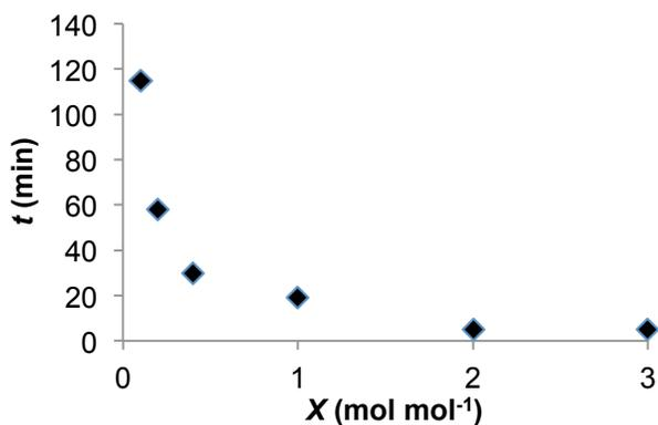
Figure 6. Decarboxylation times of phenylalanine with variable R-carvone load.
