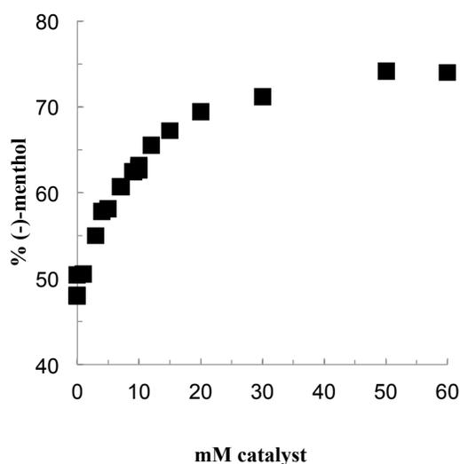
Figure 13. Product % of (-)-menthol as determined by  $^1\text{H}$  NMR is plotted vs. catalyst concentration.
