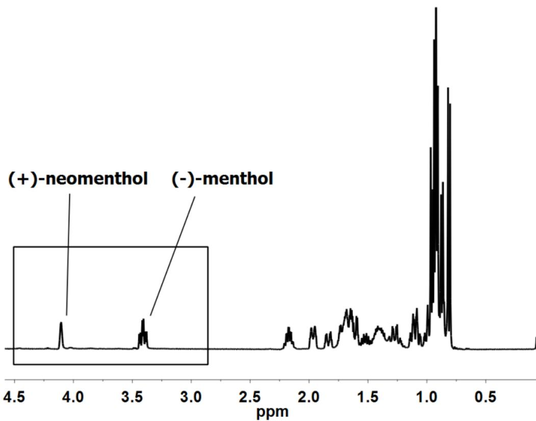
Figure 12. 400 MHz  $^1\text{H}$  NMR of a typical reduction product mixture
