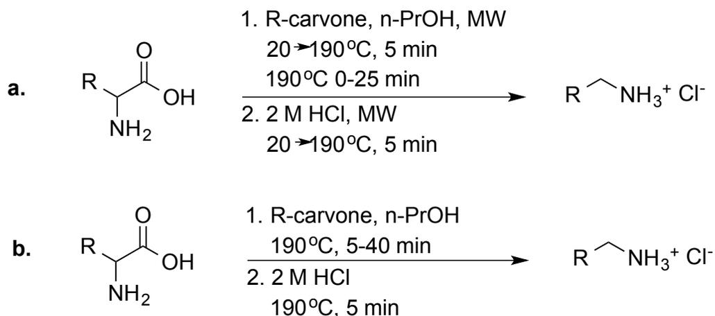
Scheme 3. Summary of microwave (**a**) and conventional heating (**b**) one-pot decarboxylation procedures
