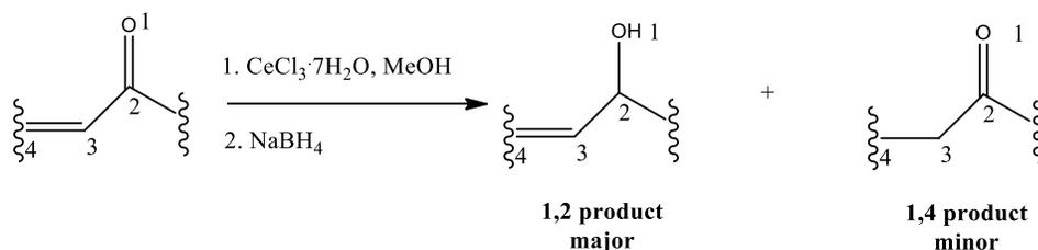
Using a Lanthanide catalyst (most commonly cerium (III) chloride heptahydrate) to activate the alcohol solvent, the Luche Reagent is rapidly formed from reaction of Sodium Borohydride with methanol solvent (Fig. 2). The alkoxyborohydride reagent formed favors reduction in 1,2 fashion more so than would sodium borohydride reduction (Fig 1).
