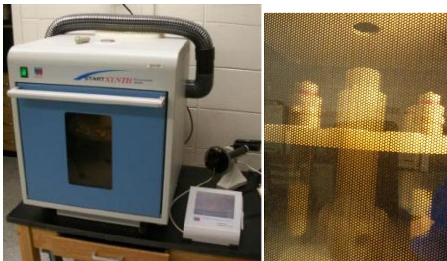
Figure 1. The Milestone START™ multi-mode microwave synthesizer
