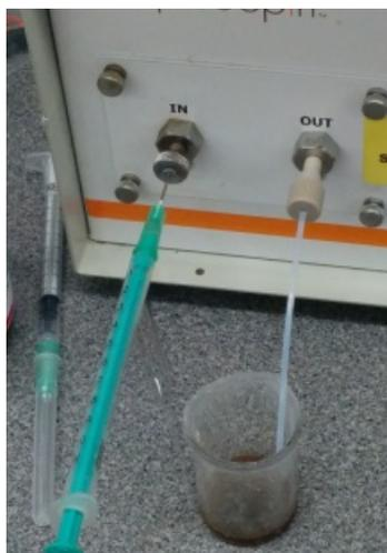
Figure 4. Syringe injection into capillary sampling region
