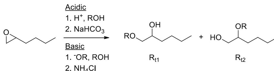
Scheme 7. Many students recognize that the major or exclusive product of the basic reactions results from addition to the less substituted position of the epoxide. This product gives rise to  $R_{t1}$  in each chromatogram.
