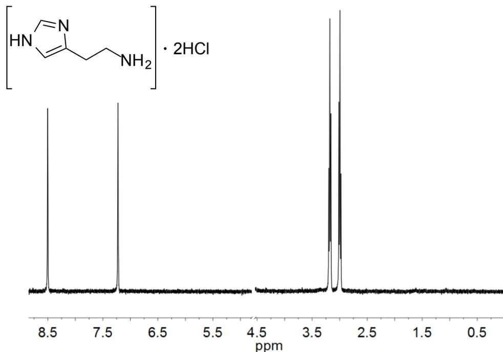
Figure 8.  $^1\text{H}$  NMR of histamine dihydrochloride with solvent  $\text{D}_2\text{O}$  suppressed
