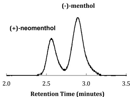
Figure 16. Student gas chromatograph of reduction product mixture is shown. Retention times for (-)-menthol and (+)-neomenthol are 2.6 min and 2.9 min respectively, and calculated product ratio is 65:35 where the expected  $^1\text{H}$  NMR calibrated value is 64:36.
