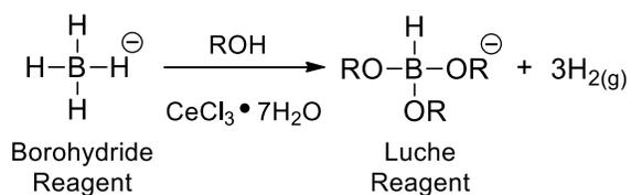
Scheme 5. Catalytic methanolysis of borohydride in forming the Luche reagent
