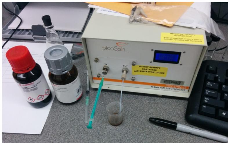
Figure 3. PicoSpin™ 45 MHz NMR Spectrometer
