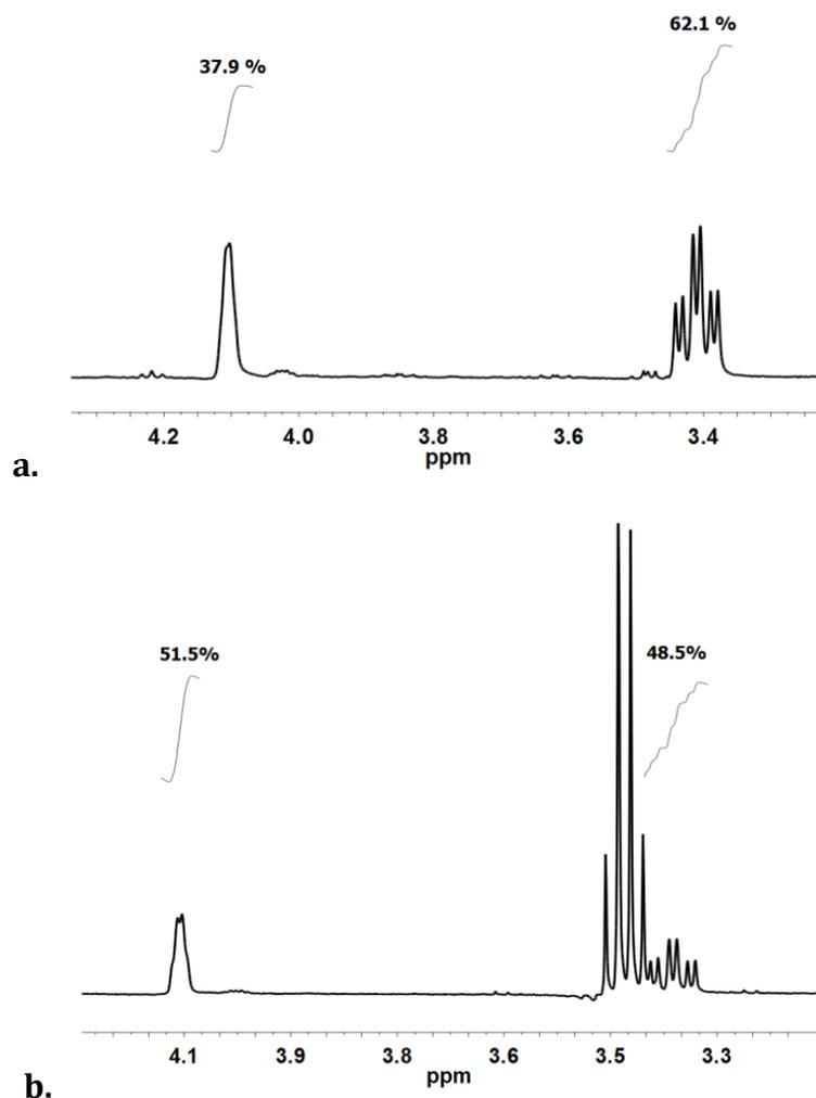
Figure 17. A high quality student <sup>1</sup>H NMR of purified product mixture is shown (a) and the analogous region of a spectrum of an impure student sample (b) with diethyl ether present are shown along with the experimental product ratios. The expected ratio of (-)-menthol : (+)-neomenthol for spectrum (a) is 64:36 ±2% and for spectrum (b) is 48:52 ±2% based on standardization results.
