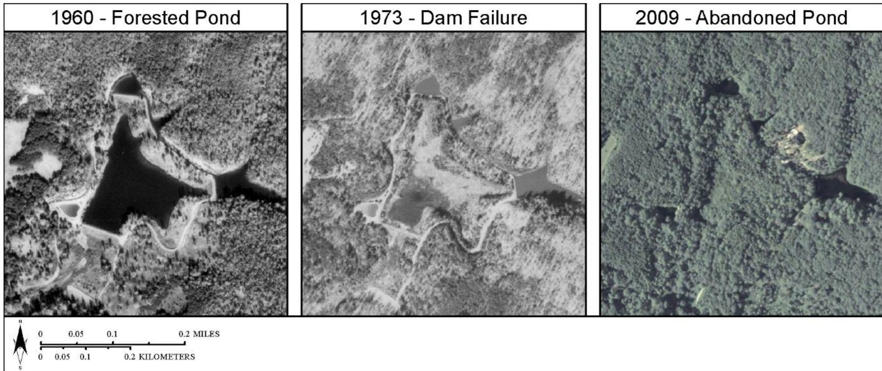
**Figure 2.9.** Example of small reservoir dam failure and subsequent reforestation.
