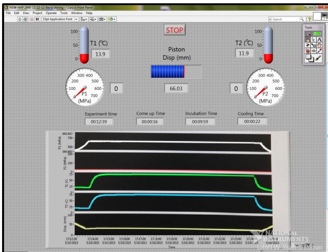
Figure A2.3. LabVIEW front panel window used to control and monitor the high pressure treatments.
