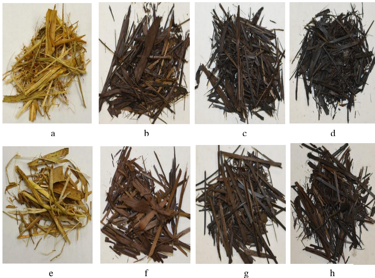
Fig.5.1 Physical change of torrefied sorghums from raw sorghums. (a) raw sweet sorghum bagasse, (b) torrefied sweet sorghum bagasse at 250°C, (c) torrefied sweet sorghum bagasse at 275°C, (d) torrefied sweet sorghum bagasse at 300°C; (e) raw energy sorghum, (f) torrefied energy sorghum at 250°C, (g) torrefied energy sorghum at 275°C, (h) torrefied energy sorghum at 300°C.
