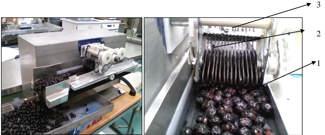
Fig. 3.1- In-house fabricated mechanical scarifier in action with side view (left) and top view (right) 1. Conveyor belt 2. Serrated rollers 3. Handle to adjust clearance between 1 & 2.
