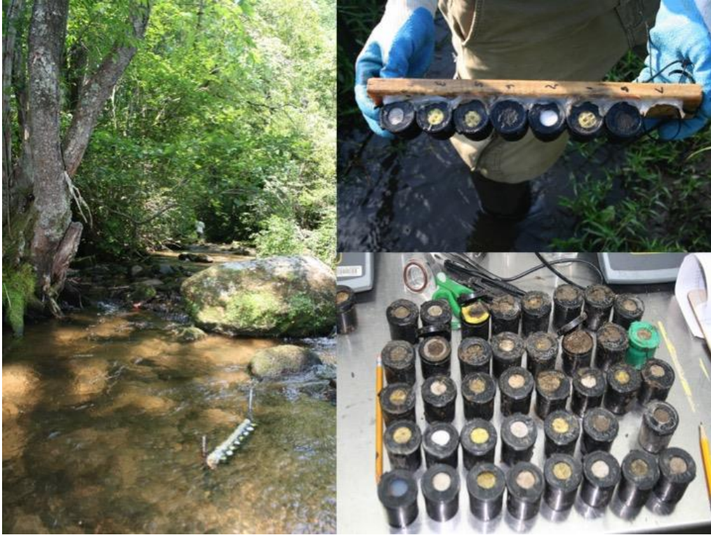
Figure 2.2. (Left) An example of a study stream showing Nutrient Diffusing Substrates array with one replicate of each nutrient treatment on both inorganic and organic substrates. Five arrays were deployed in each stream throughout a 50-meter reach. (Top Right) NDS array being removed from the stream. (Bottom Right) NDS being after deployment, note the range of conditions seen on each substrate. Photographs by J. Wood.
