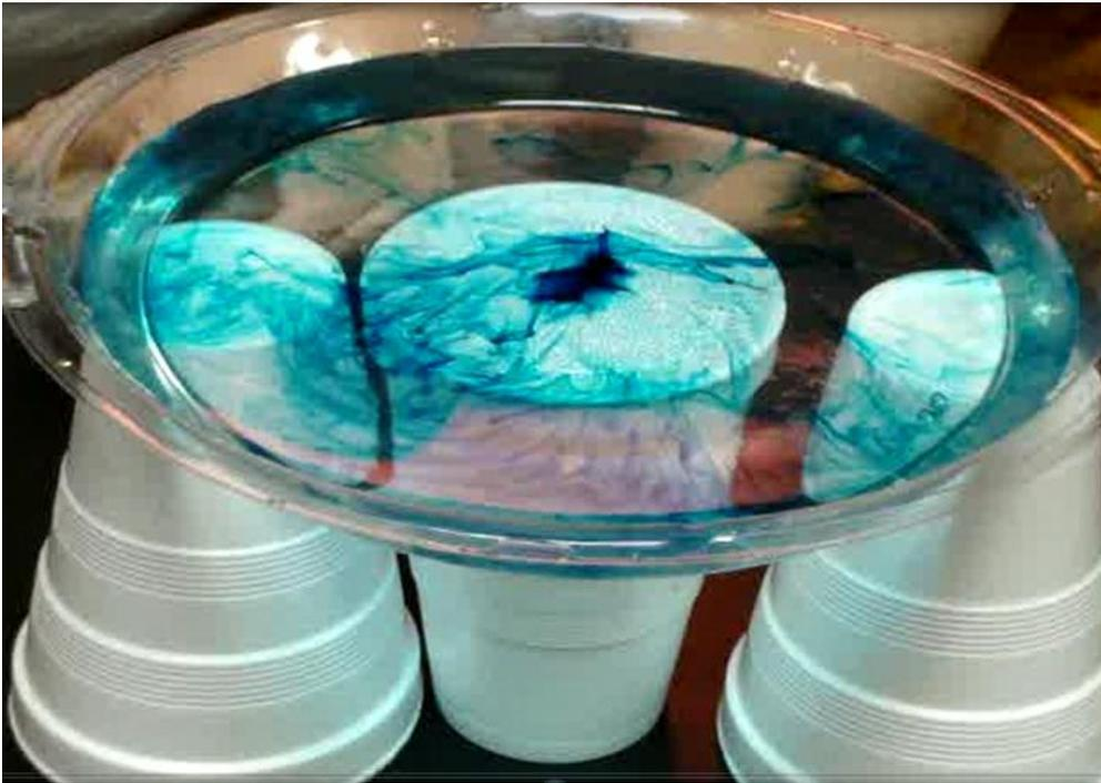
*Figure 2.10.* Lab used to show the causes of convection currents.
