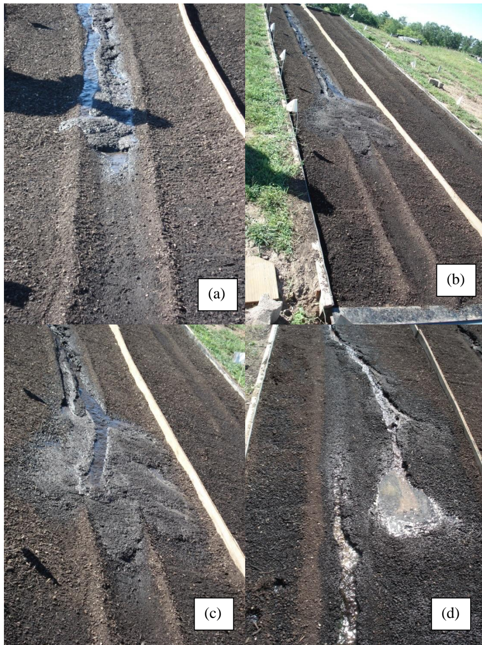
Figure 4.8. Pictures showing the micro-dams: (a) micro-dam formed across the pre-created channel, (b) micro-dam grows as solids accumulate behind it, (c) micro-dam blows out allowing flow to advance, and (d) new micro-dam was formed, encouraging more infiltration.
