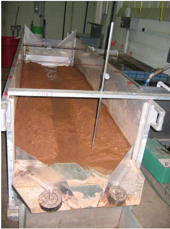
Figure 3.1 Laboratory flume for study of soil and compost erosion under concentrated flow during erosion tests of Cecil soil (Photo by Xianben Zhu, April 24, 2006).
