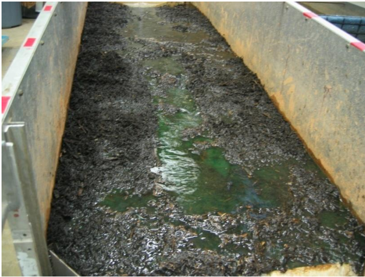
Figure 3.4 Micro-dams formed in an erosion control compost channel that blocked the flow and reduced velocity to cause infiltration and flow into the sides of the compost, resulting in the dispersal of the concentrated flow. The green color was due to a water tracing dye used to estimate channel average velocity.
