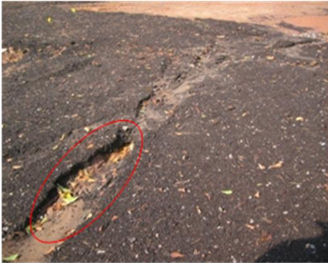
Figure 2.1 A picture showing a rill forms in compost applied on a construction site with slope of 3.5 percent. (Photo by Xianben Zhu)
