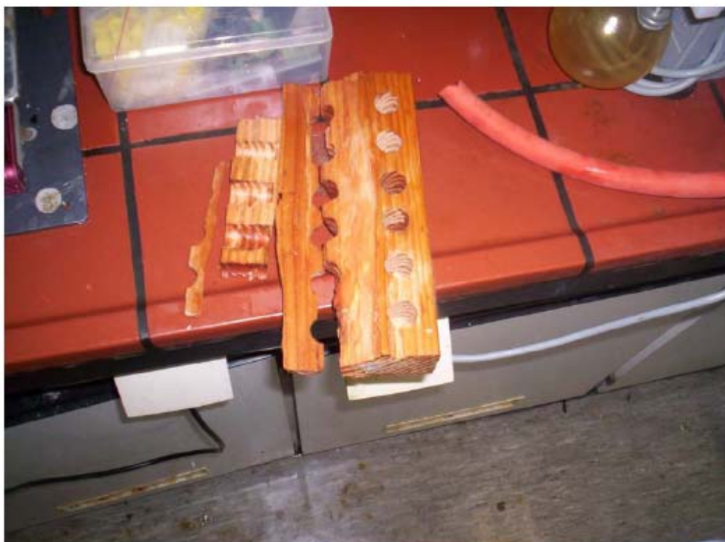
Figure 9. The glass side shield of a fume hood and an oak rack destroyed by a detonation of [\text{C}_1\text{mim}][\text{ClO}_3] .
