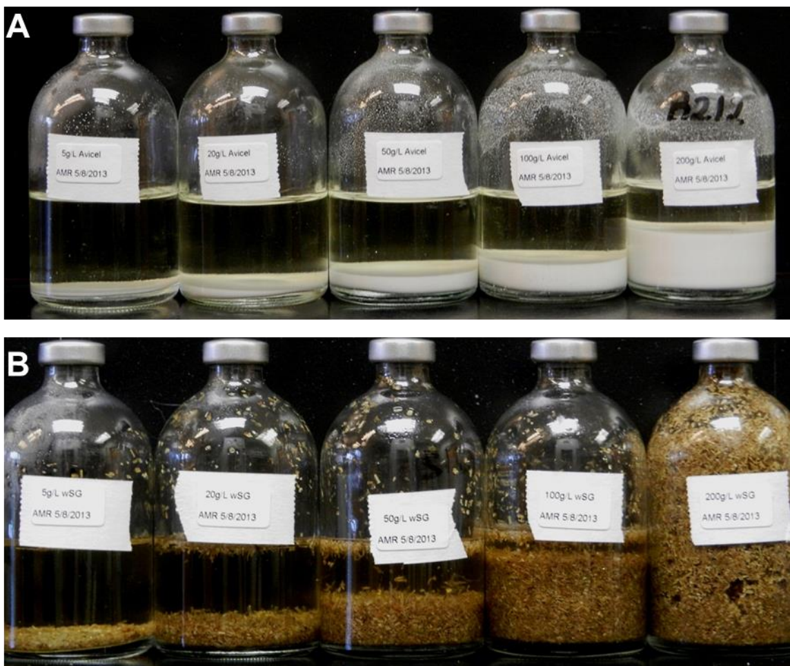
Figure 2.2 Growth of C. bescii on different loads of cellulose and untreated switchgrass. 5, 20 and 50 and 200 g L -1 of cellulose (A) and the same concentrations of untreated switchgrass (B) in closed cultures.
