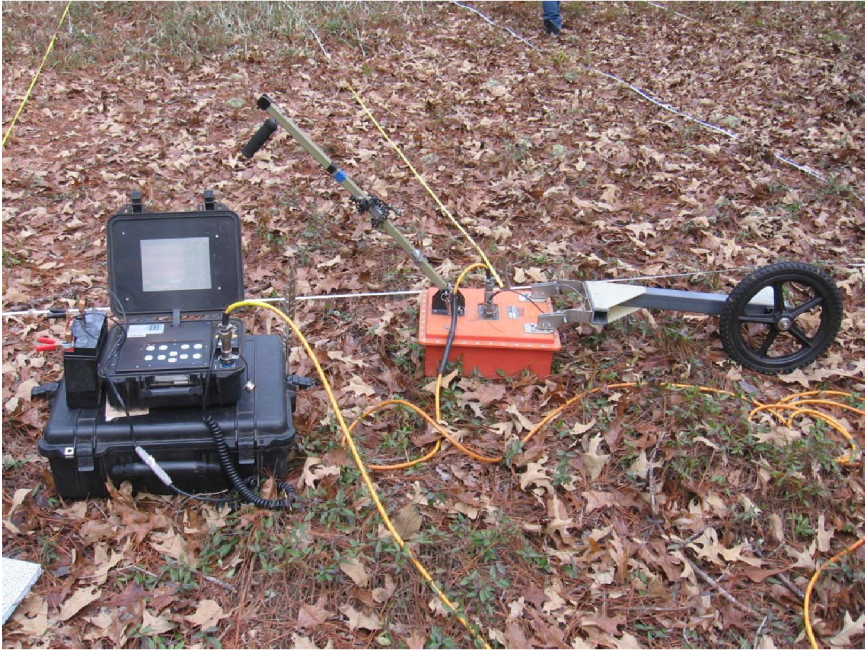
Figure 3.3: SIR2000 GPR control unit with 500 MHz antenna connected to the survey wheel.
