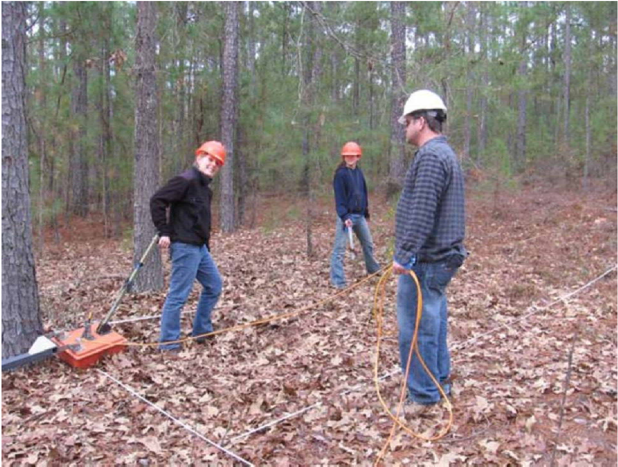
Figure 3.4: GPR surveying in action at Plot 1 with UGA personnel from the Geology Department and the Warnell School of Forestry and Natural Resources.
