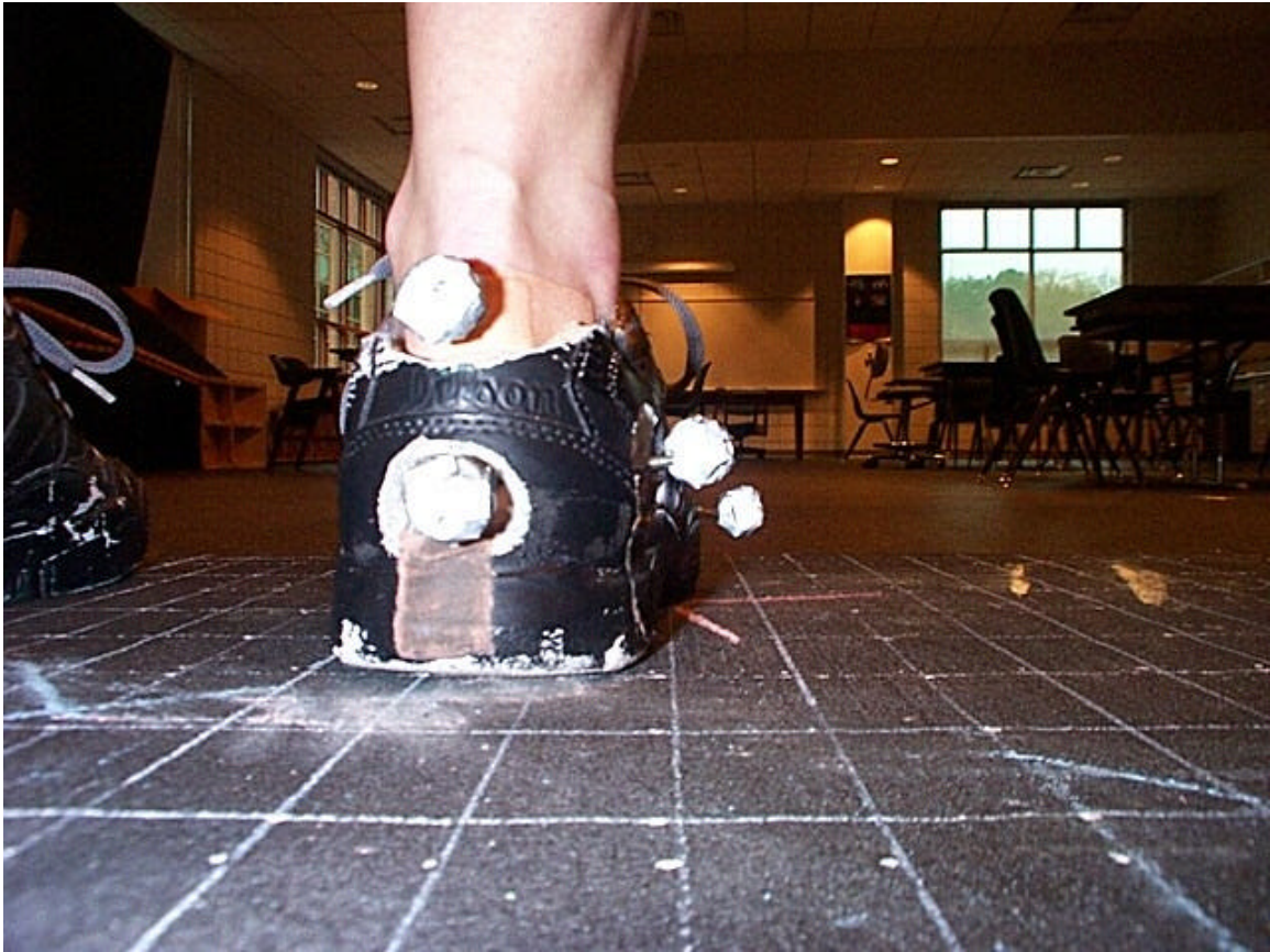
Figure 8. Posterior view of the foot segment markers comprised of the T-nut, machine screw, reflective ball and shoe as applied to the participant.
