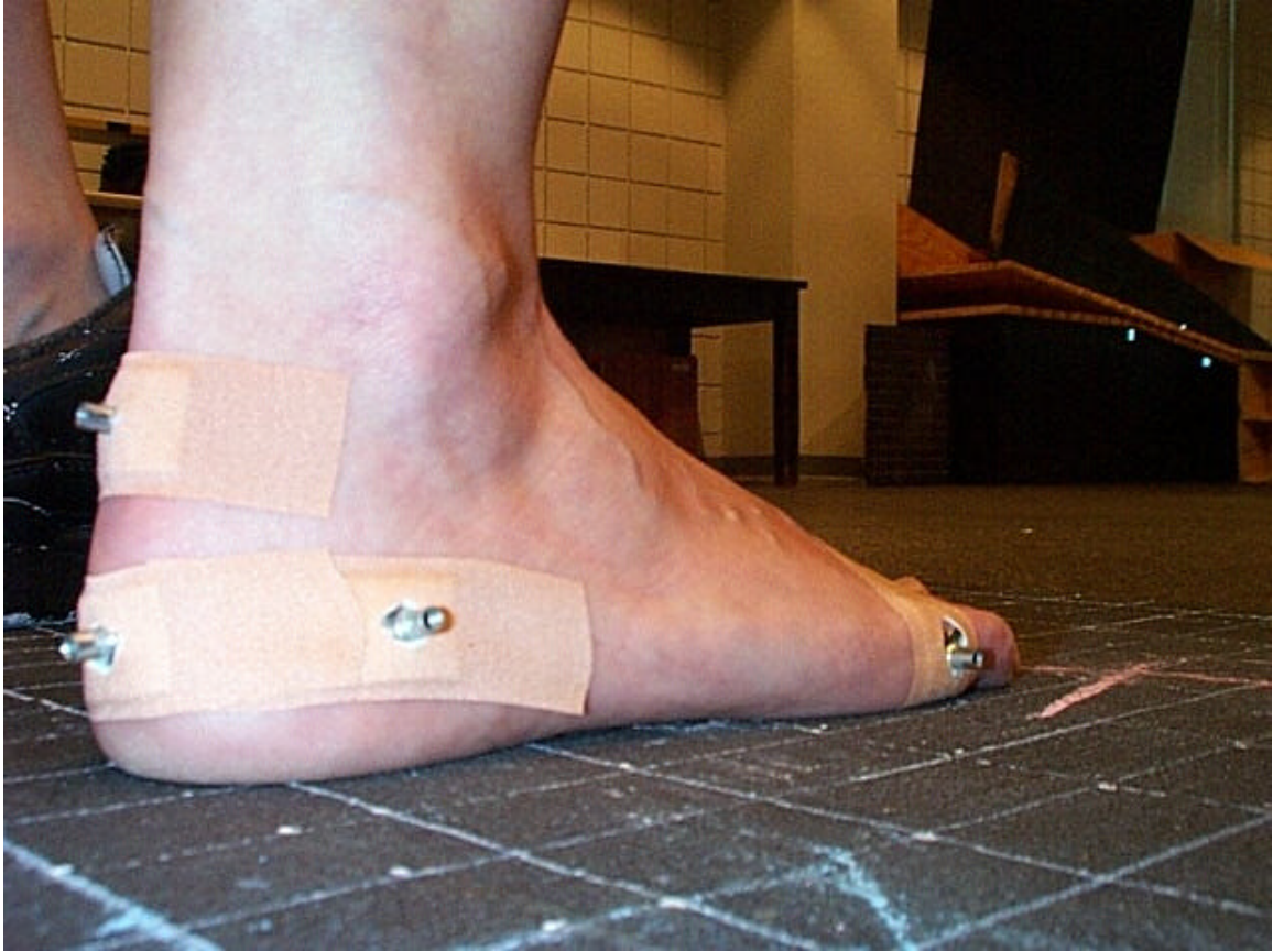
Figure 6. Angled lateral view of T-nut application to the skin of a participant for the foot segment markers.
