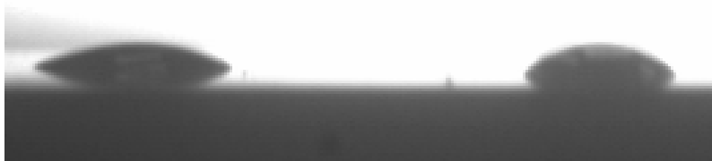
Figure 3.6: Water Droplets on 4-Vinylpyridine End-functionalized Nb Polymer Brush Surface After Acid Treatment.
