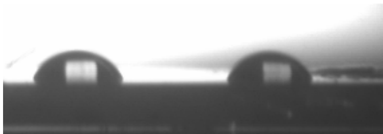
Figure 3.5: Water Droplets on Styrene End-functionalized Norbornene (Nb) Polymer Brush Surface After Acid Treatment.
