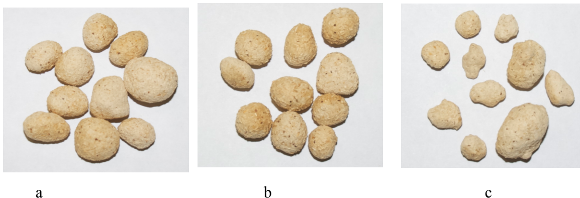
Figure 4.2. Pine granules formed from different binder concentrations: a) 2.5% b) 5%, c) 7.5%
