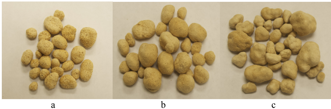
Figure 4.4. Pine granules made with various mean powder particle sizes: a) 397 \mu\text{m} , b) 225 \mu\text{m} , c) 135 \mu\text{m}
