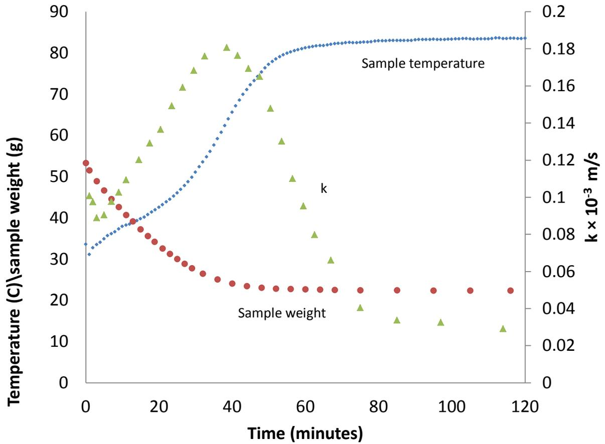
Figure 4.3. Temperature, sample weight and characteristic drying coefficient (k) change as a function of time during vacuum drying: T=100°C, L= 2.3mm, and P=20 torr.
