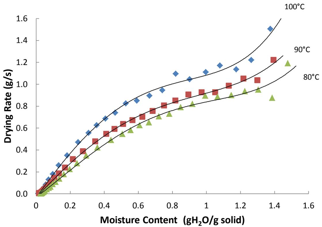
Figure. 4.4. Drying rate during vacuum belt drying of tortilla chips.  $L = 2.3\text{mm}$ ,  $P = 20\text{ torr}$ .  $A = 28.26\text{ cm}^2$ .
