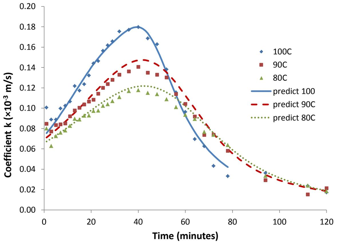
Figure. 4.6. Characteristic drying coefficient ( $k$ ) as a function of time and fit by a two term Lorentzian model.
