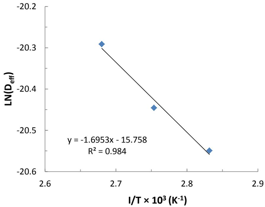
Figure. 4.5. Effect of temperature on the average drying effective diffusivity of the vacuum drying of tortilla chips
