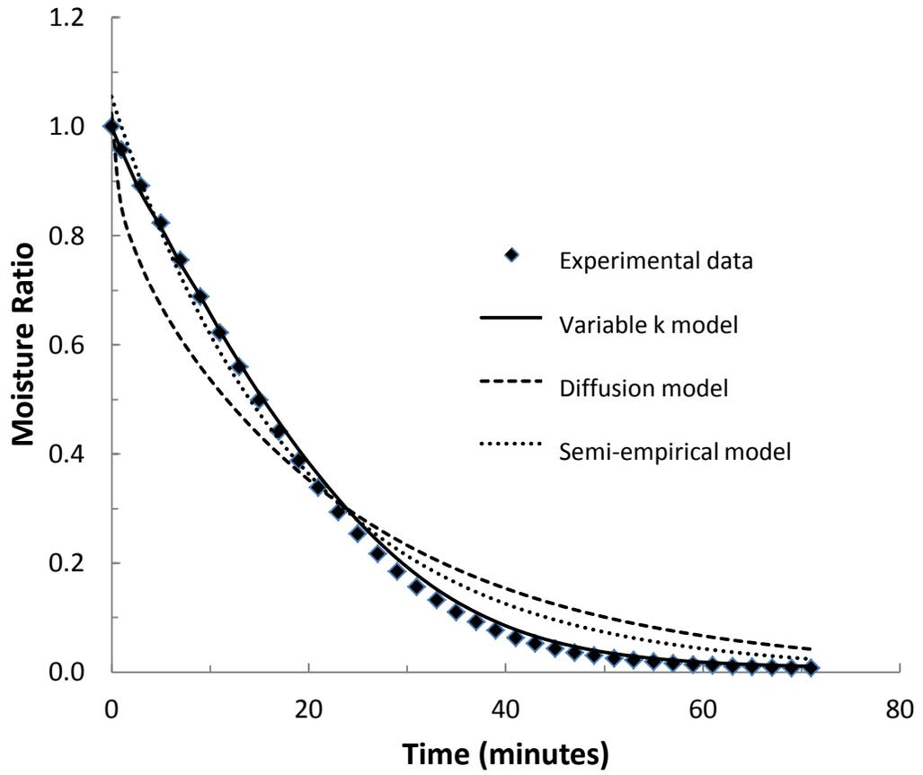
Figure. 4.7. Model fits to drying rate data at  $T=90^{\circ}\text{C}$ ,  $L=2.3\text{mm}$ ,  $P=20$  torr.
