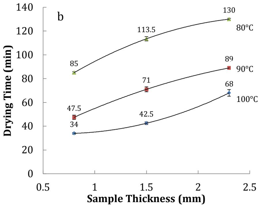
Figure 5.2. Relationship of drying time (time to reach 3% moisture) with (a) heating temperature and (b) chip thickness. Pressure: 20 torr.
