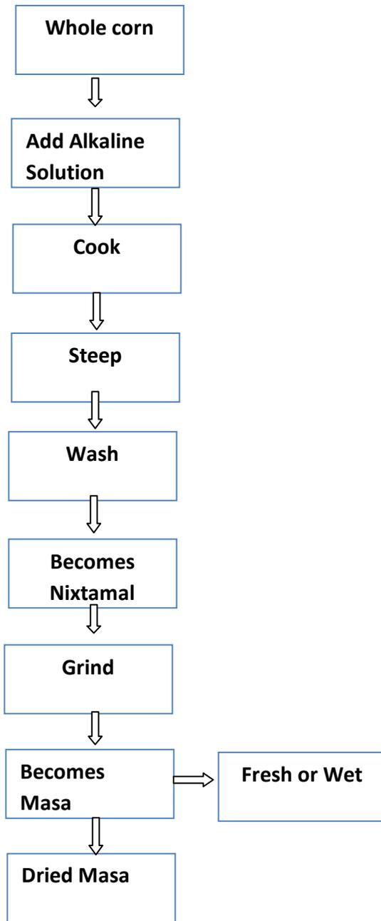
Figure 2.2 Nixtamalization and masa process
