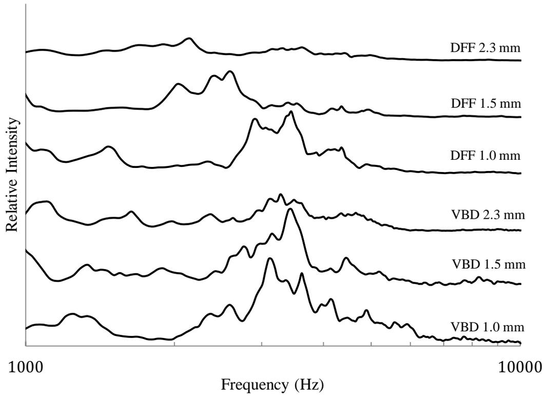
Figure 3.3: Frequency spectrum of CVD and DFF chips of various thicknesses during fracturing in the Crisp Fracture Rig
