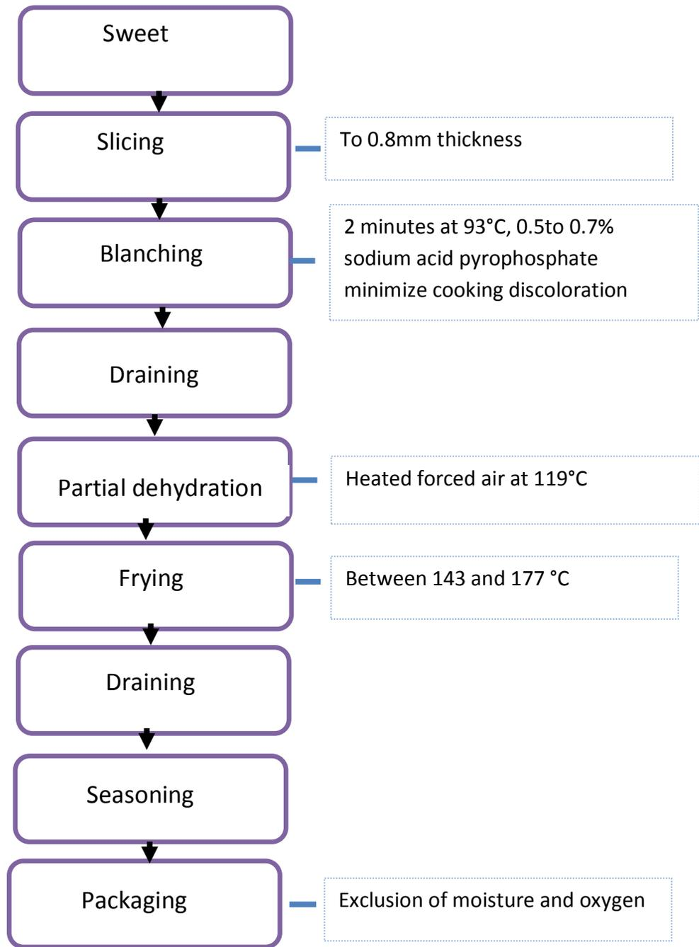
Figure 2.3 Process of preparing sweet potato chips
