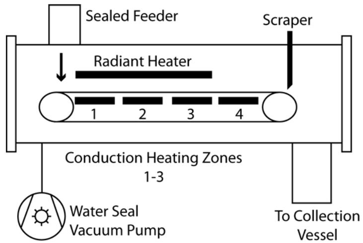
Figure 3.1: Schematic diagram of the continuous vacuum belt drier.
