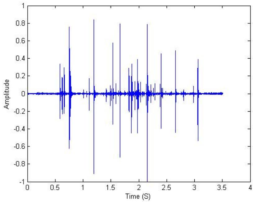
Figure 3.2: Sound profile during fracturing of CVD chips in the Crisp Fracture Rig
