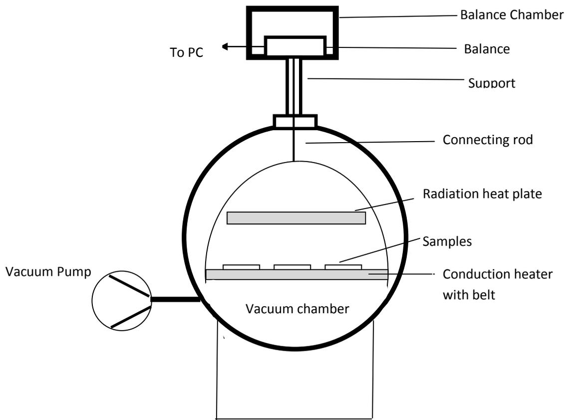
Figure . 4.1. Continuous vacuum belt dryer with attached balance for determining drying rate.
