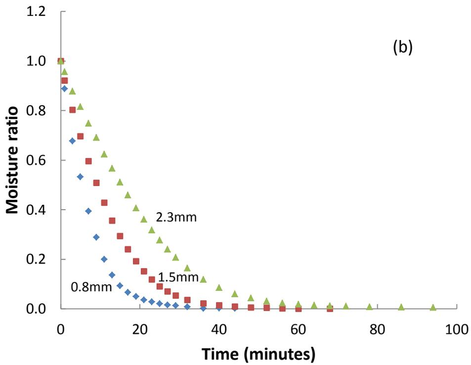
Figure.4. 2. Vacuum drying of tortilla chips as a function of: a. temperature ( $L=2.3\text{mm}$ ) b. thickness ( $T=90^\circ\text{C}$ ).
