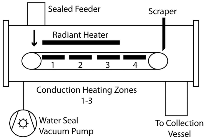
Figure 6.1: Schematic diagram of the continuous vacuum belt drier.
