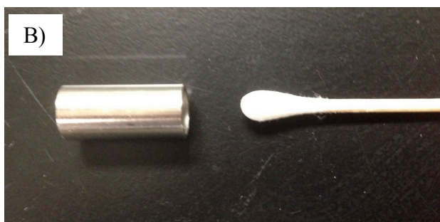
Figure 2.14. Stainless steel tube size and eight swabbing directions inside the tube. A: Tube placed horizontally and vertically compared to the size of a quarter coin. B: Tube and cotton tip used for swabbing. C: Eight swabbing directions on the inner surface of the tube sample.
