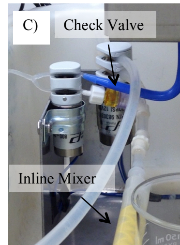
Figure 2.7. Prototype 4, including continuous dilution and mixing to slow down the growth rate of biofilm. A: Flow system layout, two bottles system. B: Whole system looks. C: Valves used to control the mixing operation.
