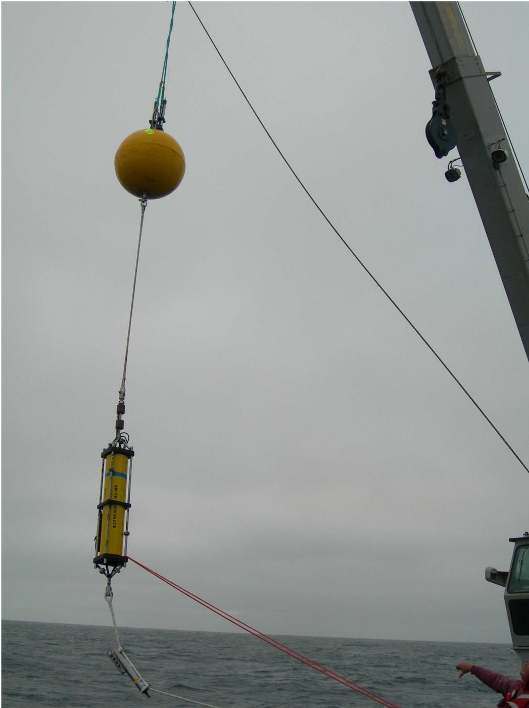
Figure 2.15: Photo showing the deployment of the Transmitter mooring from the RV Atlantis (photo courtesy of D. DiIorio).
