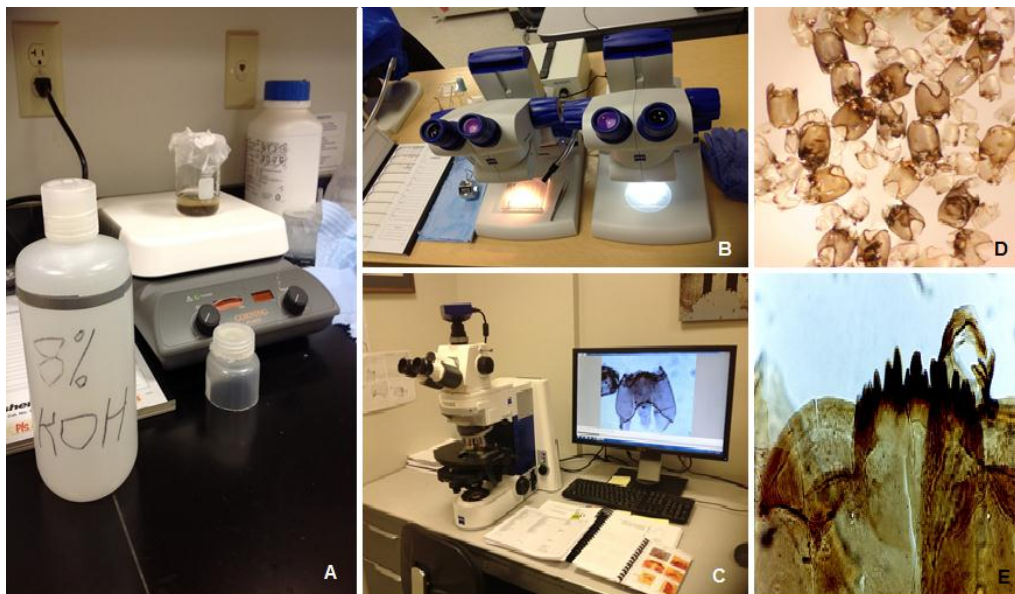
Figure 3.4 Procedure for extracting and identifying subfossil midge remains. (A) Sediment is treated with an 8% KOH solution and heated at 50°C for \sim 30 minutes to facilitate the break-up of colloidal matter. (B) A dissection microscope at 50X and a Bogorov plankton counting tray are used to separate the chironomid head capsules from the sediment matrix. (C) The chironomid remains are permanently mounted on slides in Entellan for identification. (D) Chironomid head capsules prepared for making permanent slides. (E) A photograph of a Chironomus head capsule at 400x.
