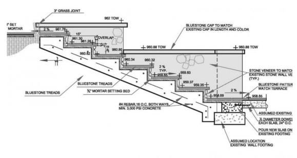
STAIRS TO POOL SECTION ELEVATION
