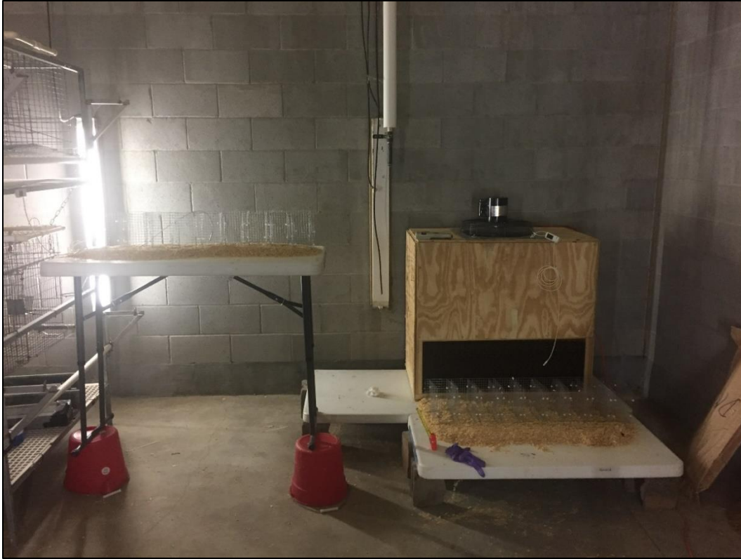
Figure 1. Air movement treatment setup. Eight individual cells served as the control group (left) with no air movement where eight individual cells served as treatment group (right). The fan generated 0.5 or 1 m/s air movement over the treatment cells.
