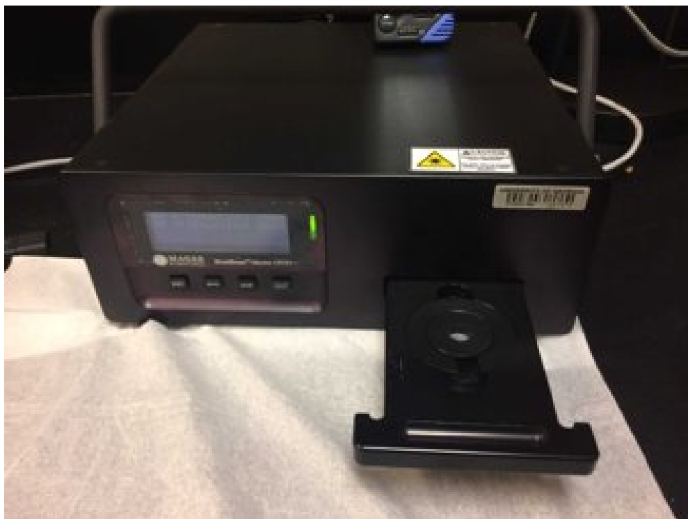
Figure 3. 1 Image of the SootScan OT 21 Transmissometer. The image is of the SootScan that was used at UGA. The cartridge slots are pulled out so that the blank filter can be scanned. The image shows the 15mm cartridge with a filter in place.
