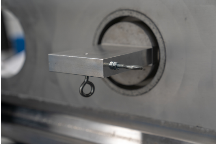
Figure 3.10. View of the test block secured to the force balance [1]
