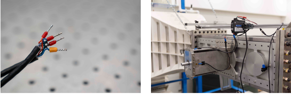
Figure 3.3. (a) Ferrules and (b) force balance wired to signal conditioner [1]
