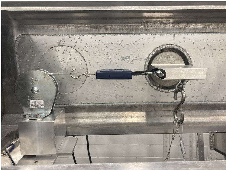
Figure 3.11. Side view of the pulley system to support calibration weights
