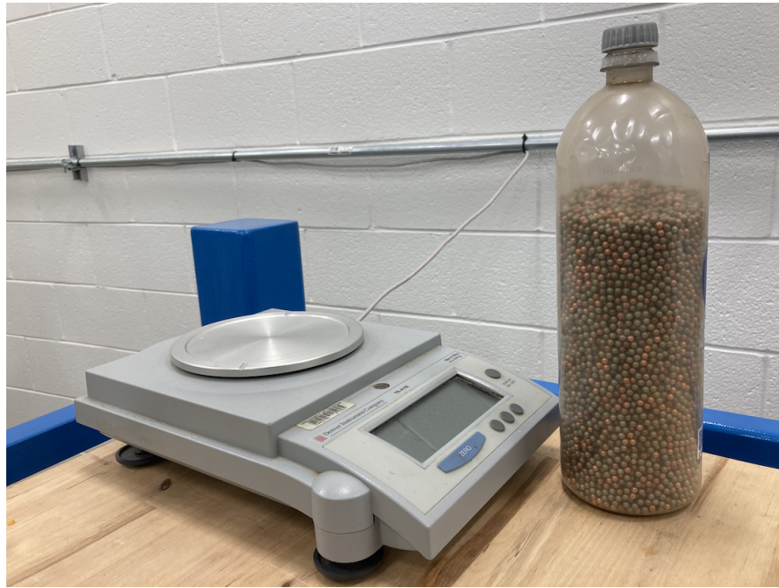
Figure 3.12. Precision table scale and steel BB's used to load the balance
