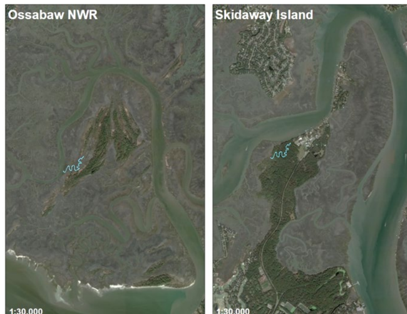
Figure 23: Location and morphology of tidal creek traced from an island within Ossabaw National Wildlife Refuge, then superimposed onto the Skidaway campus in the area of the proposed tidal creek restoration.
