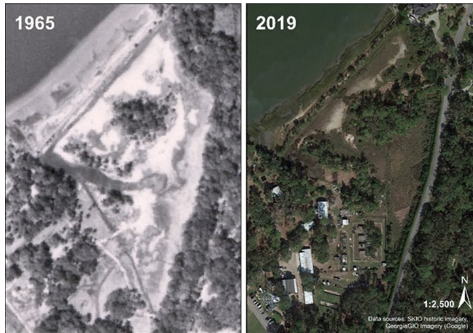
Figure 33: 1965 aerial imagery shows inlet before bulkhead and shortly after installation of berm (left) (SKIO historic imagery 1965). Current aerial imagery shows berm and bulkhead restricting flow into/out of tidal inlet (right).
