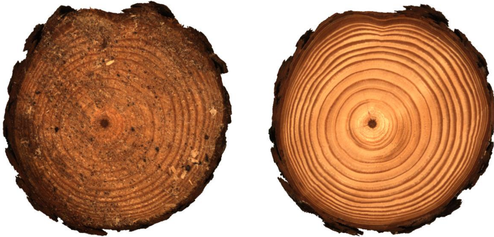
Figure 2.1: Image showing typical surface quality of a chainsaw cut wood disk (left). The image on the right shows the same disk after surface preparation.
