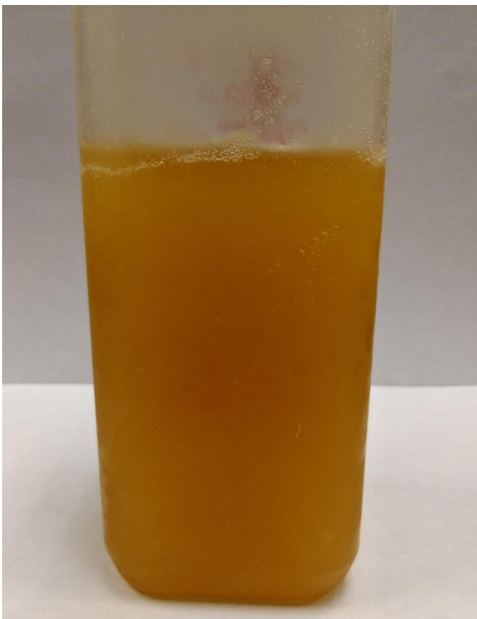
Fig. 3.2 Liquid hydrolyzed jellyfish collagen (LHC) before dialysis
