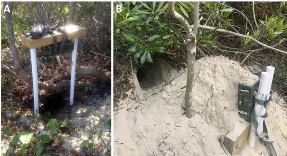
Figure 3.2. Example of the two types of camera setups used during study. (A) Setup with camera above burrow, (B) Setup with camera across from burrow. Cameras set up across from the burrow have increased risk of being blocked or covered by excavated soil.
