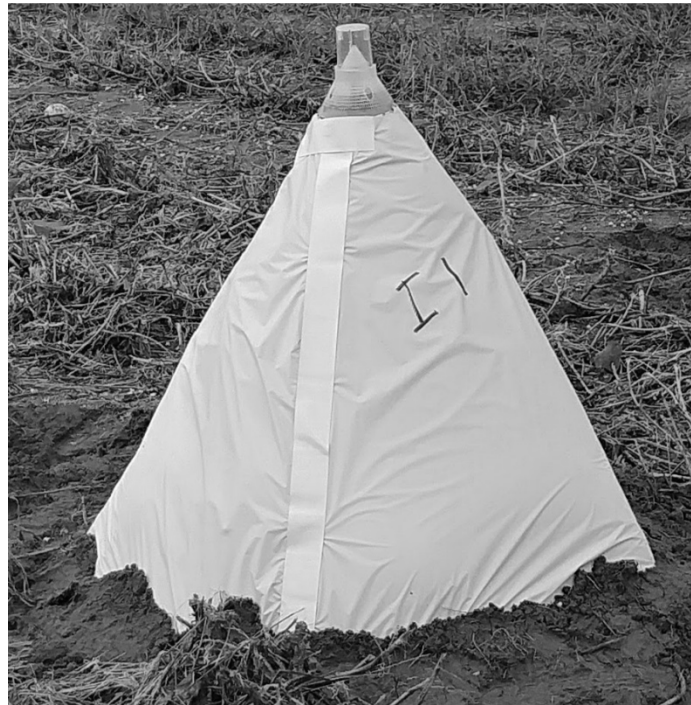
Figure 4.1. Below is an example of the Covered Modified Heliothis Traps used to monitor cowpea curculio adult emergence.
