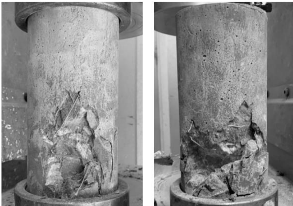
Figure 35: Localized Failure Observed During Compressive Strength Tests
