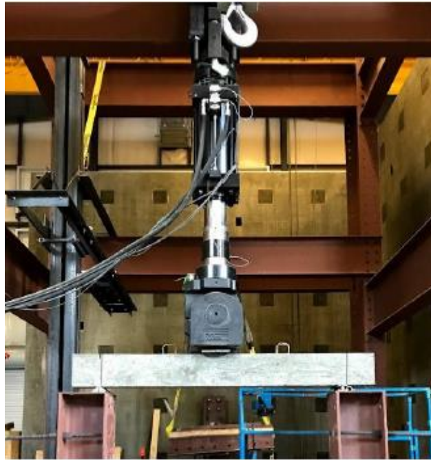
Figure 27: Static Beam Test Setup
