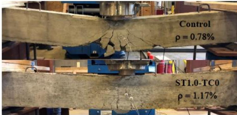
Figure 19: Anterior View of Fractured Impact Beam Specimens (Lopez, 2018)
