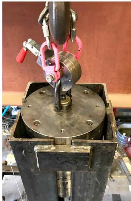
Figure 18: Drop Weight at Top of Steel Sleeve (Lopez, 2018)
