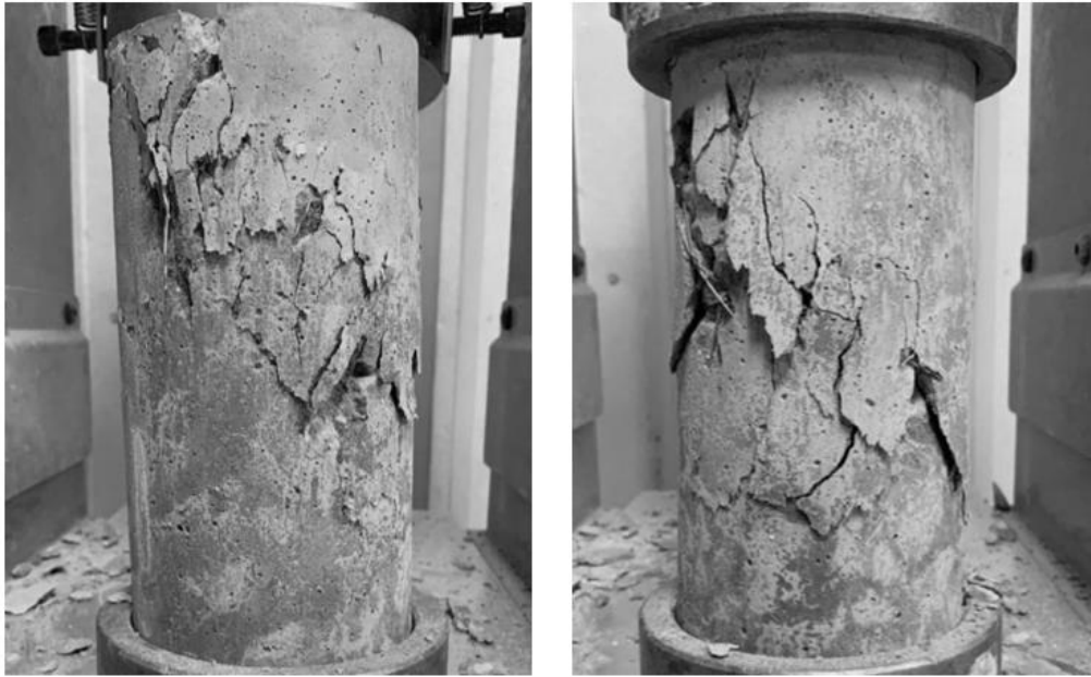
Figure 34: Crushing Failure Observed During Compressive Strength Tests
