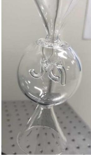
*Figure 5: Image of the jet-stirred reactor. Direction of flow is downward.*
