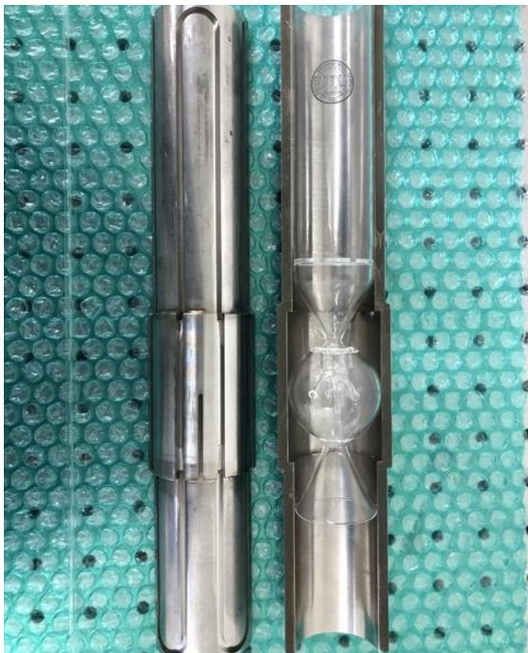
*Figure 29: Reaction volume of the JSR inside its main heaters. A clear gap is shown as the geometry changes.*
