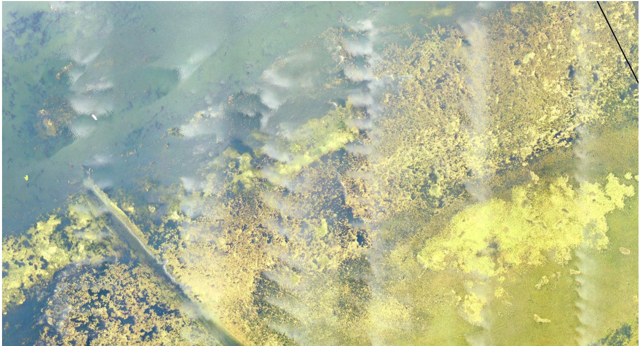
Figure 3.4: Striping in an orthomosaic from cloud-induced overexposure
