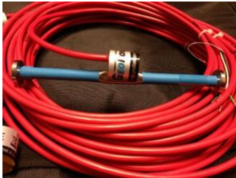
Figure E.1 – Embedded vibrating wire strain gauge.
