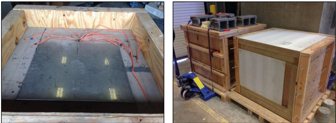
(d) putting top lid on (e) adding top insulation and formwork and tightening the specimens
