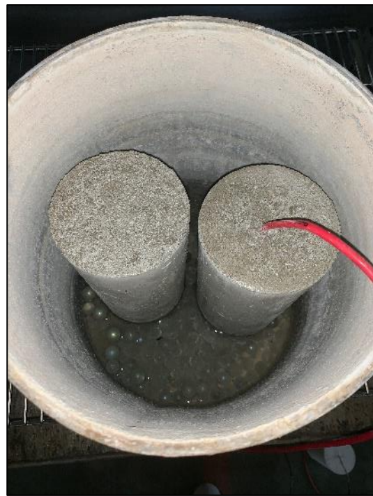
(b) marble spheres under the cylinders inside the bucket
