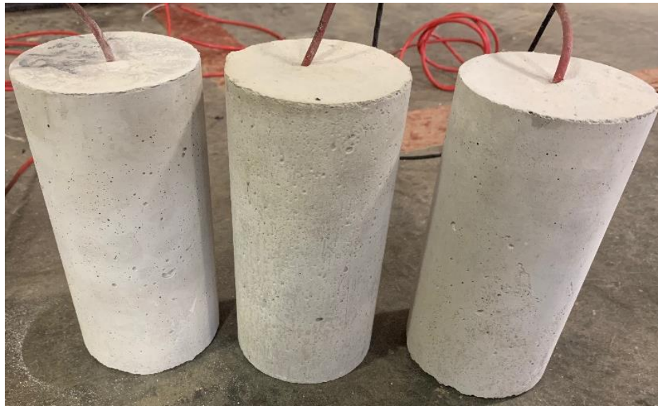
Figure E.4 – Concrete cylinders after being exposed to elevated temperature.
