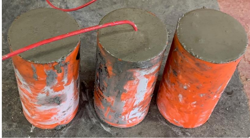
Figure E.2 – Casting concrete specimens with strain and temperature gauge.
