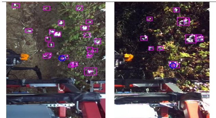
Figure 6.9. Boll detection using tiny YOLOv3 and ZED camera. Left image: cloudy day, Right image: sunny day.
