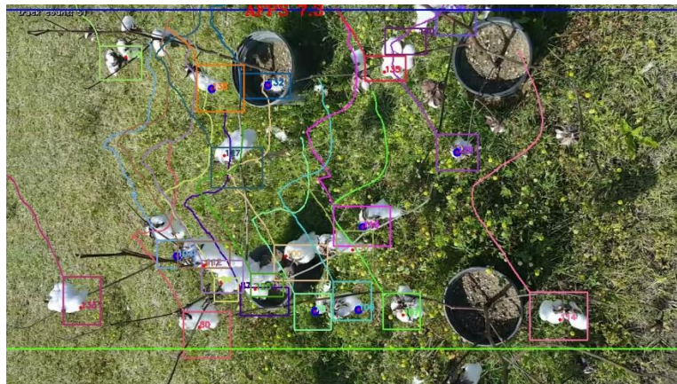
Figure 3.6. Tracking of the cotton bolls. The lines indicate tracklets, which is the path the bolls were detected across different frames. The green line is the line which the boll which was tracked from at least previous 4 frames will be counted
