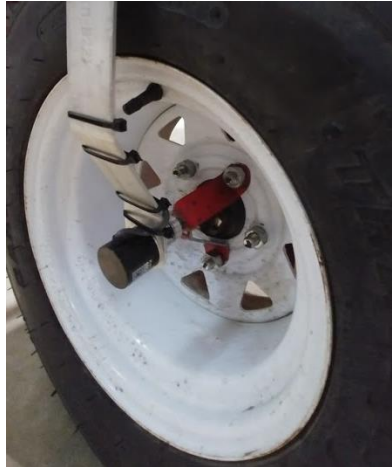
Figure 6.4. Encoder installed on the front tire of the rover to provide input pulses which indicates how far the rover has moved from one point to another
