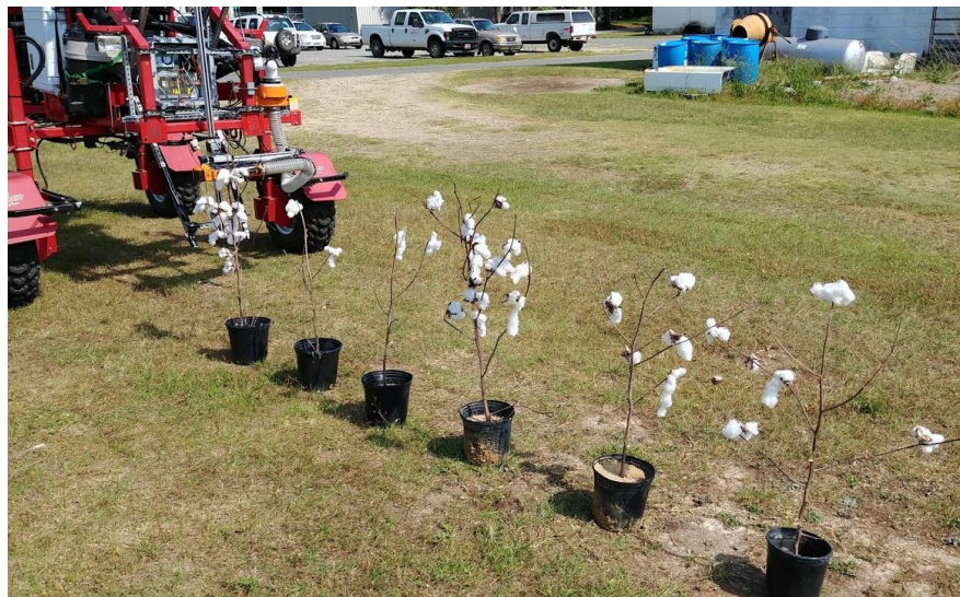
Figure 6.21. The experiment was set up at UGA grounds to test the robot on picking the bolls on a simulated environment consisting of six potted cotton plants.
