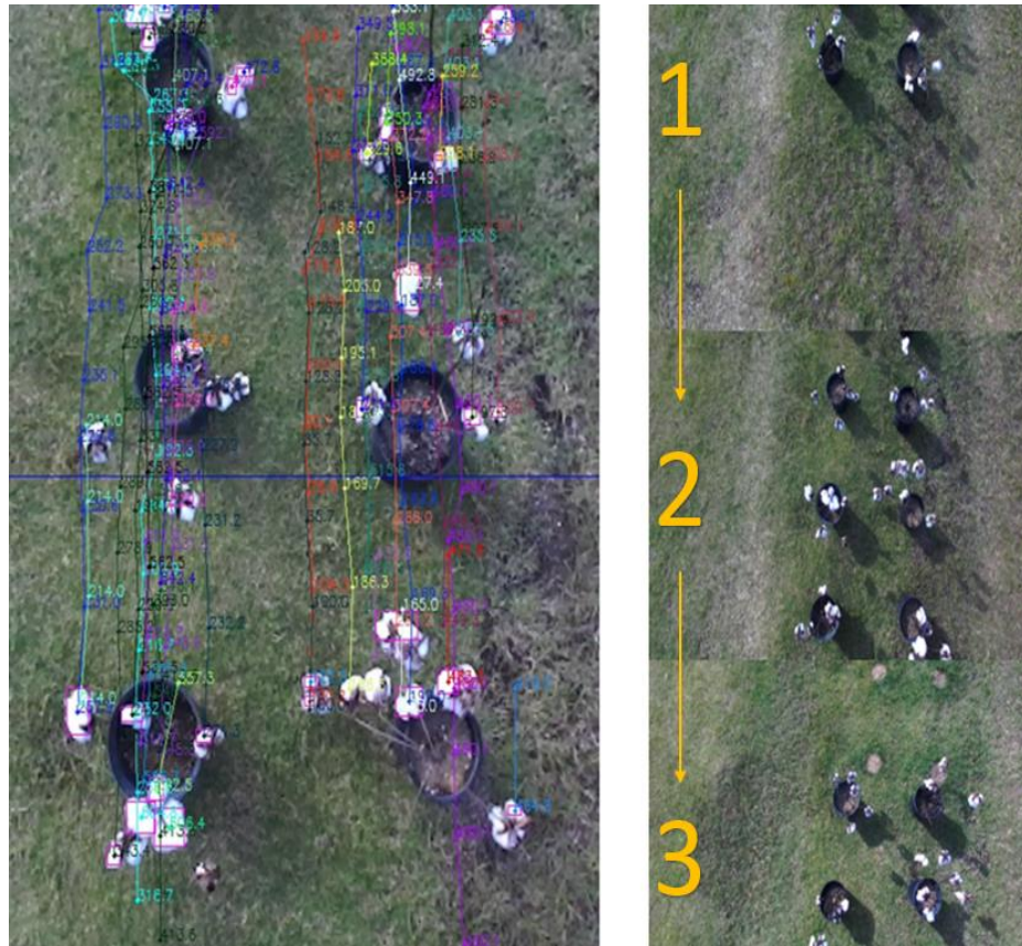
Figure 4.9. Left image show processed boll position and tracking of the boll while the right images show a series of 3 image frames acquired from the moving camera.
