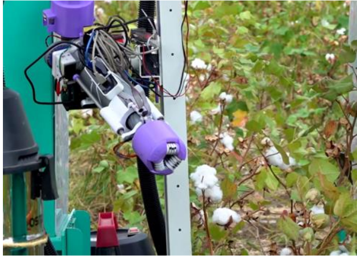
Figure 2.9. Green Robot Machinery (gRoboMac) manipulator trying to get the cotton boll (source: www.grobomac.com ).
