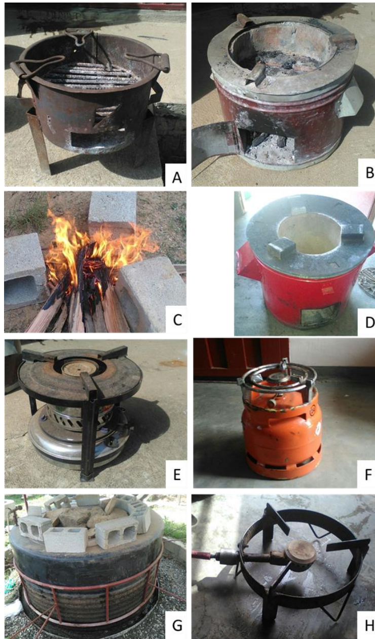
Figure 2: Possible EvaKuula fuel/burner combinations evaluated. A - regular charcoal stove, B - improved charcoal stove, C - three stone stove, D - improved firewood stove (Rocket Lorena stove type), E - kerosene stove, F - butane cylinder with burner, G - biogas digester floating dome type, with block on top to increase pressure under the dome, and H - biogas burner connected to the biogas digester.
