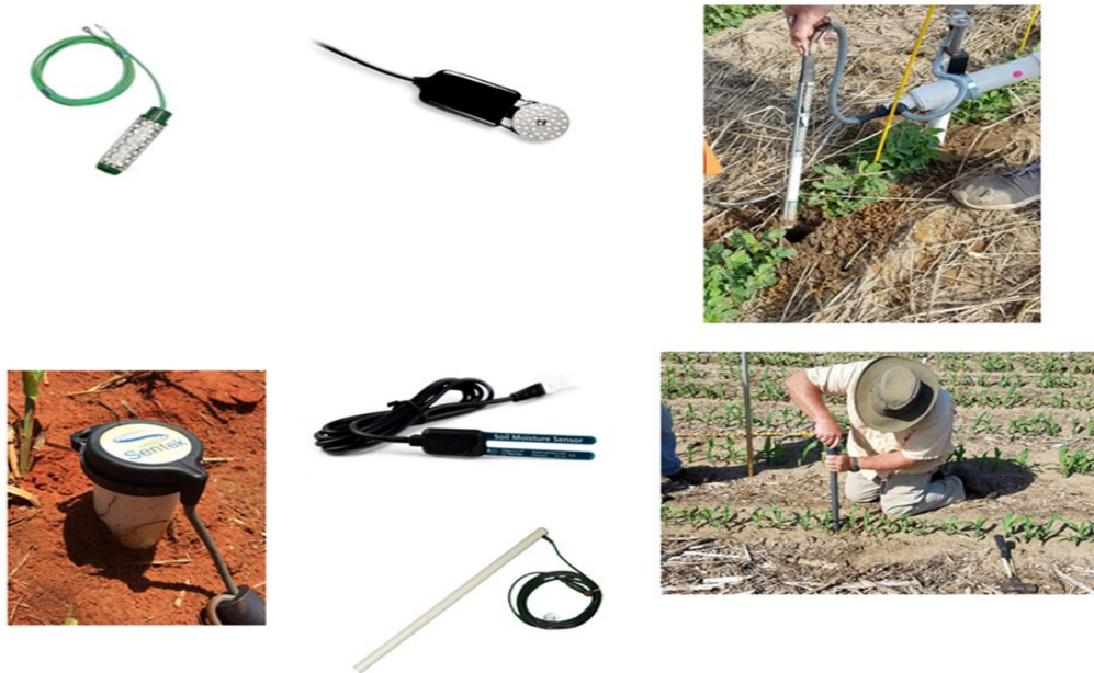
Figure 4: Sensors based system including tensiometric system (Top) and capacitance system (Bottom).
