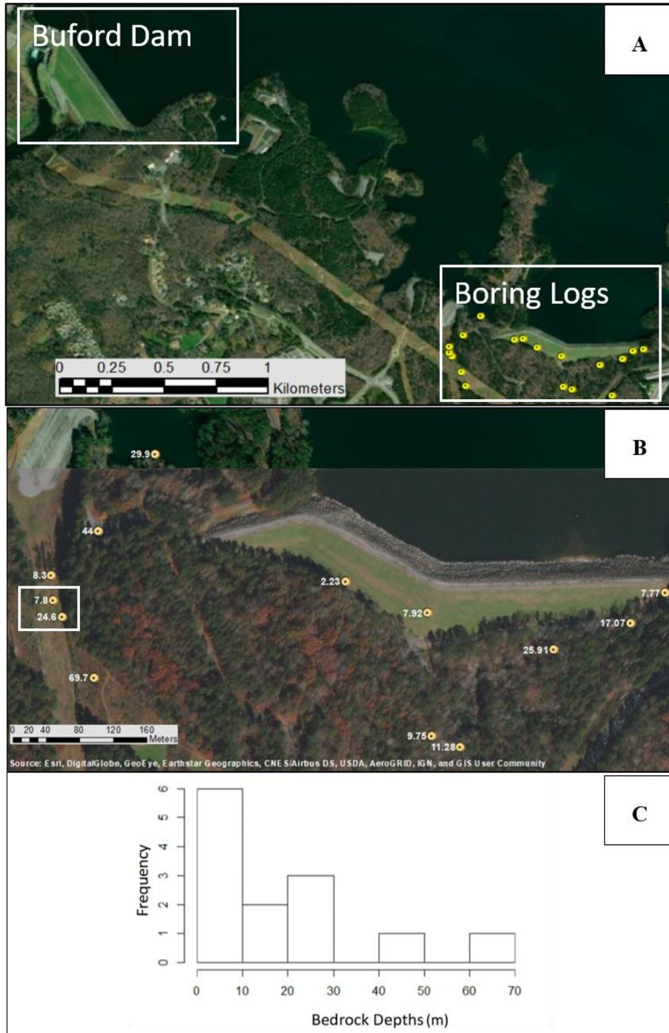
Figure 3.1. Image A shows the locations of the boring logs in respect to Buford Dam, in Buford, GA. B is a blow-up of the area containing the boring logs and shows the depth to bedrock, in meters, as reported by the Us Army Corps of Engineers. In the highlighted box in B, depth to bedrock changes by 17 m with a 10 m distance. Image C presents the same data as a summary of the frequencies of the depths to bedrock.
